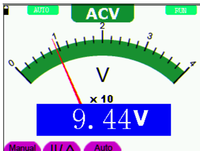
Figure 26: AC Voltage Measurement
