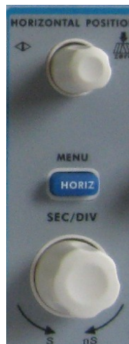
Fig. 4-13 Horizontal Control Zone
