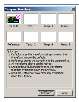
**Default** – it stores the waveforms on the Waveform Window by default.
