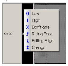
Only one trigger (channel) can be set as Rising Edge ↑, Falling Edge ↓ or Change ↑.
