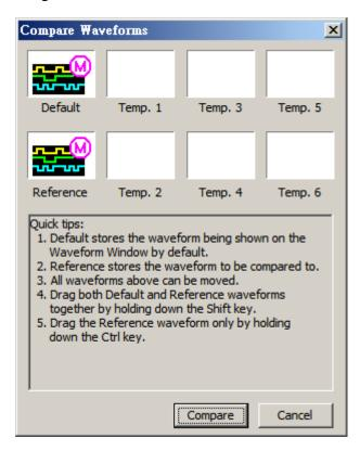
Then click Compare to return to the LA Viewer window and open the second waveform file (Test2.law), you will see the Test1 as the Reference waveforms and the Test2 file as the Default waveforms.
