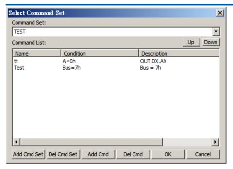
Add Select Command Set button from Toolbar → Toolbar Buttons and click it to show the dialog box below; there are 4 quick settings - add command set (Add Cmd Set), delete command set (Del Cmd Set), add command (Add Cmd) and delete command (Del Cmd). The command set must be saved as \*.CMS, similar to the Windows Excel file \*.CSV, so you can edit the command set in Windows Excel and load it into the LA Viewer.
