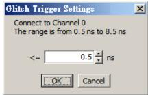
ONLY Channel 0 (default) can be the glitch trigger channel. Parameter range:  $0.5 \sim 8.25$  nanosecond (ns) with a 0.25 ns interval.
