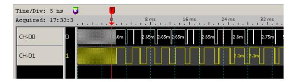
If the logic analyzer is stopped when capturing data, then the waveform on the right of the waveform window is invalid and will be marked as dots.
