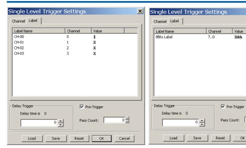
Double click or right-click on the label name, channel, or value of any single channel to set its value (x is the default) as the menu below, but ONLY one channel can be set as Rising Edge  $\uparrow$ , Falling Edge  $\downarrow$ , or Change  $\updownarrow$ .
