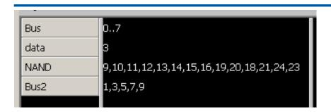
The first column is the Label name, which can be in English characters or with alphabetic numbers; the second column is the Channel number which can be "0..7" to represent a bus form channel 0 to channel 7 or in a number "2" to represent the channel 2.
