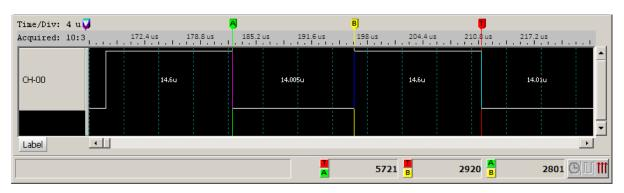
Click any cursor button to display the cursor menu below to choose any two buttons to measure the frequency, timing, or sample clocks between them.
