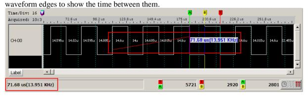
Scroll the mouse wheel to zoom in/out waveforms centered on the mouse cursor.
