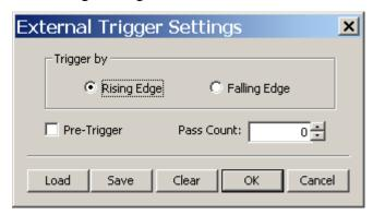
The TravelLogic series support all four trigger conditions: Rising Edge, Falling Edge,
