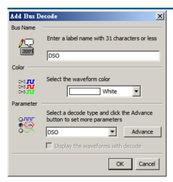
Set more parameters like Bus Name (DSO), Color (White), Parameter (DSO), and check Display the waveforms with decode, then click Advance to show the DSO Stack Settings dialog below.
