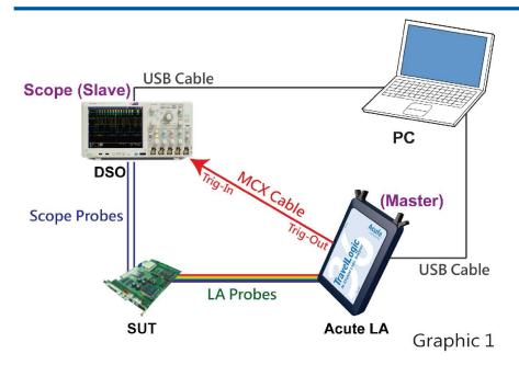
Connect the logic analyzer (Trig-Out) with the DSO (Trig-In or Ch4 for Tektronix MDO4000 serial) over a MCX-BNC able for the Tektronix/Agilent/GW Instek DSO (MCX-MCX cable for Acute DSO); connect the DSO with the PC over an USB or Ethernet cable.
