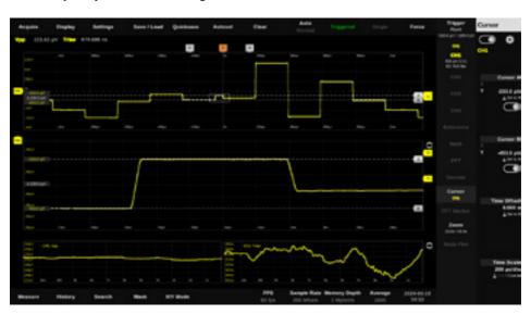
The screenshot shows triggering on a signal detail as small as 220  $\mu$ V (!). In the zoom view (centre), you can see the signal detail with a resolution of 50  $\mu$ V/div, and the measurement trend charts (below) show the time progression of the Vpp voltage and the rise time of this signal detail.
