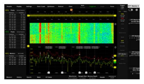
For the screenshot, a BicoLog antenna without amplifier was connected directly to the input of the Magnova. At the top you can see the signal in the time domain, at the bottom the amplitudes in the frequency range LF to 800 MHz with spectrum, average and max hold display and in the centre the time progression of the spectrum in a waterfall display. Some peaks and marker values are shown in tabular form on the left.
