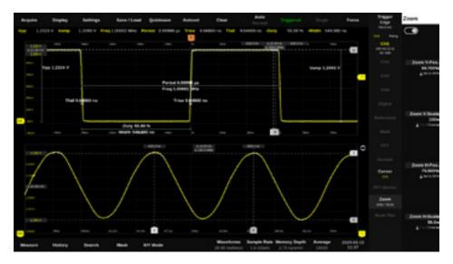
The screenshot shows a 100x vertical zoom on the only 12 mVpp large sinusoidal 100 MHz noise interference on a square wave signal (1 MHz). Thanks to the 16-bit system architecture and the powerful zoom function, the signal and the noise, which is a hundred times smaller, can be measured and displayed in detail.
