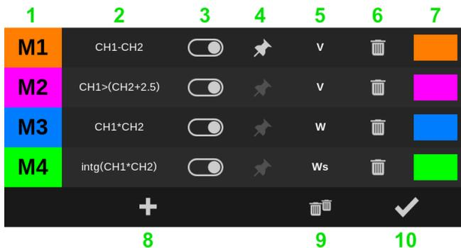
1. Each math channel has a designation (M1, M2, ...) which is also displayed on its marker to the left of the measurement curve display area. You can change the order of the list by dragging the number.
