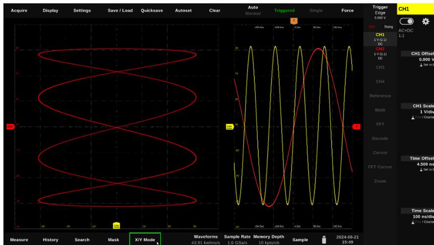
To activate the XY display, please tap on "X/Y Mode" at the bottom of the screen, set the channels in the dialog that then appears and tap on the slider to activate or deactivate the display.
