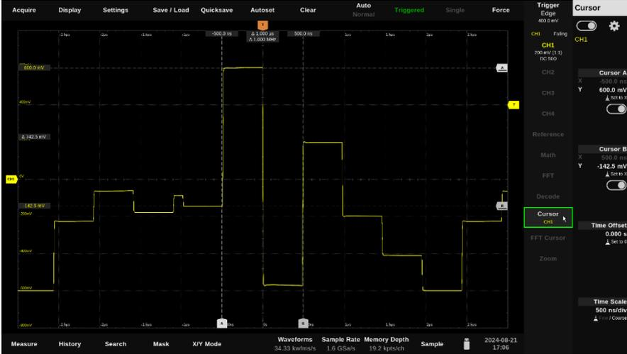
Tap on "Cursor" in the control selection to show the cursors. Tap on the gearwheel that appears to the left to open the cursor settings window.
