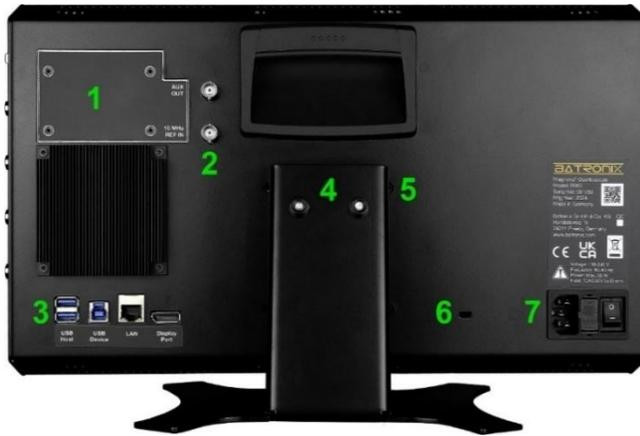
1. Cover for retrofitting the Magnova function generator module. Also used as a maintenance opening for easier access to the battery for the built-in real-time clock. A screwdriver with a TX10 head is required to loosen and tighten the screws.
