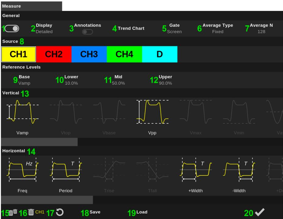
1. The display of the measured values can be switched on and off using the slider.
