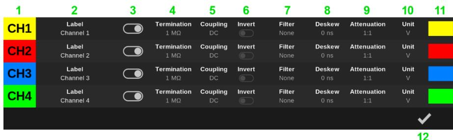
1. Each channel has a designation (CH1, CH2, ...) which is also displayed on its marker to the left of the measurement curve display area.
