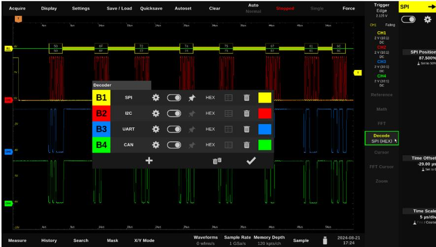
Tap on "Decoder" in the control selection and then on the plus sign that appears to the left of it to create a new decoder.
