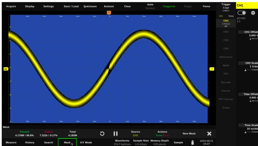
To display the mask test control bar, please tap on "Mask" at the bottom of the screen. You can close it tapping again.
