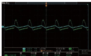
CV 50V low speed mode: it's obvious to find vibration phenomenon
