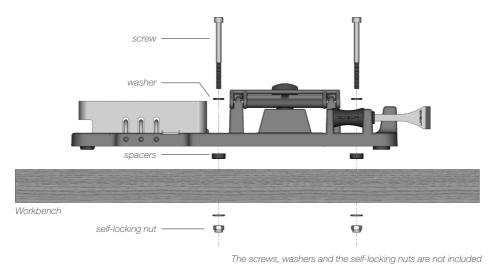
To fix the CT-SA in place, put the spacers (Ref. 0014899) between the stand and the workbench. This means you protect the stand's rubber feet from wear and tear.
