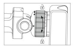
You can lock or unlock the lateral rotation mechanism by turning the fixing wheel a quarter.
