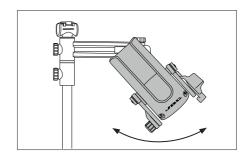
The movement allows a rotation between -90° and +90°.
