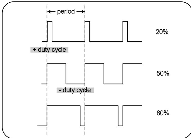
**Figure 3-10** Positive and negative duty cycle measurements.
