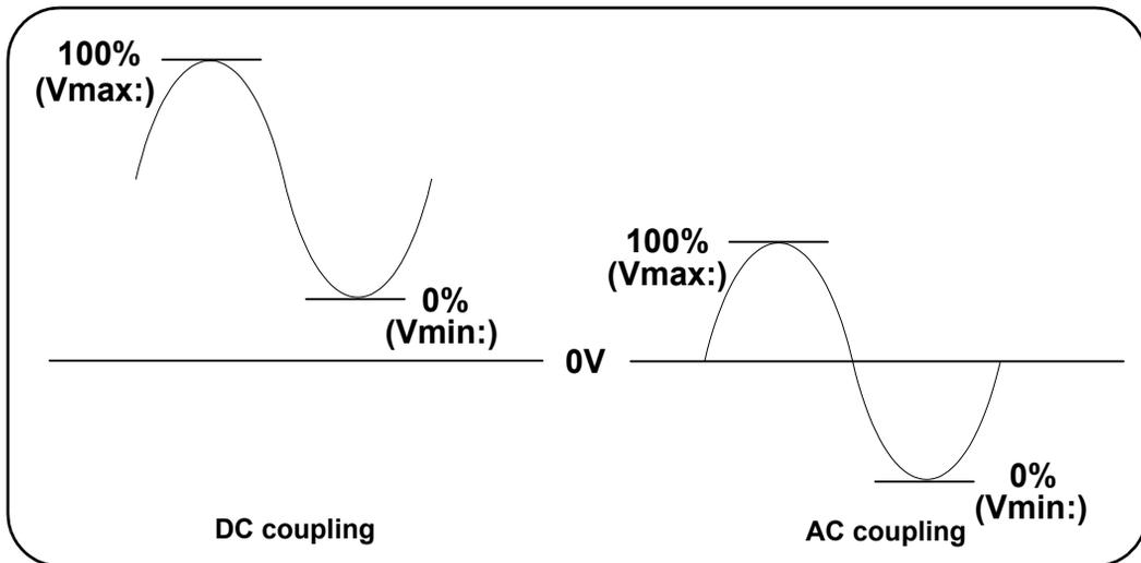
**Figure 4-5** Input coupling and relative threshold levels.
