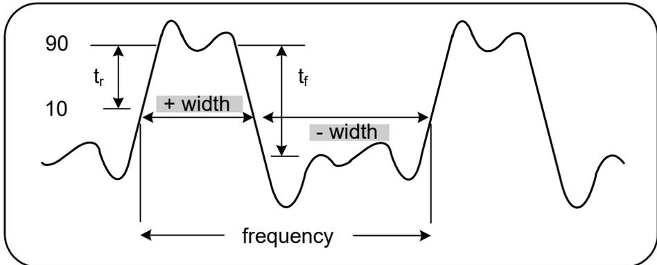
**Figure 3-9** Positive and negative pulse width measurements.
