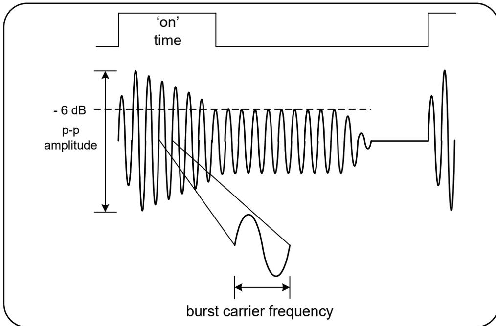
**Figure 5-6** Burst carrier frequency (-6 dB threshold).
