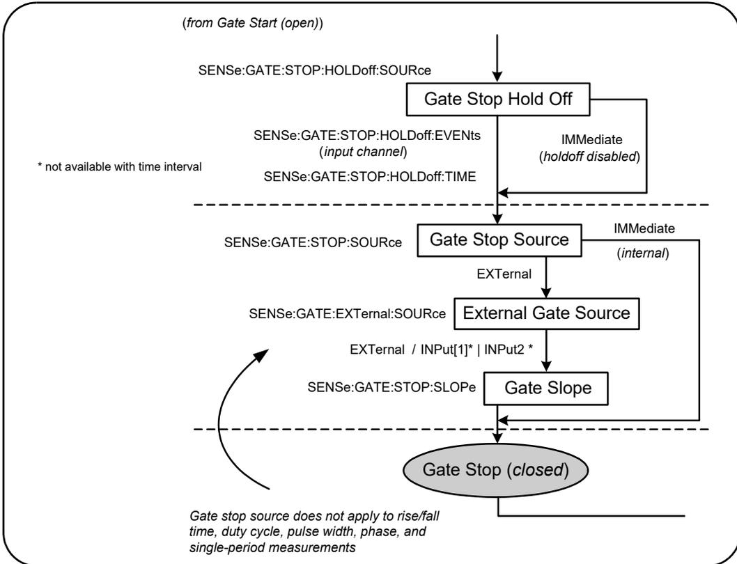
Figure 5-9 Gate stop hold off and gate stop sequence.
