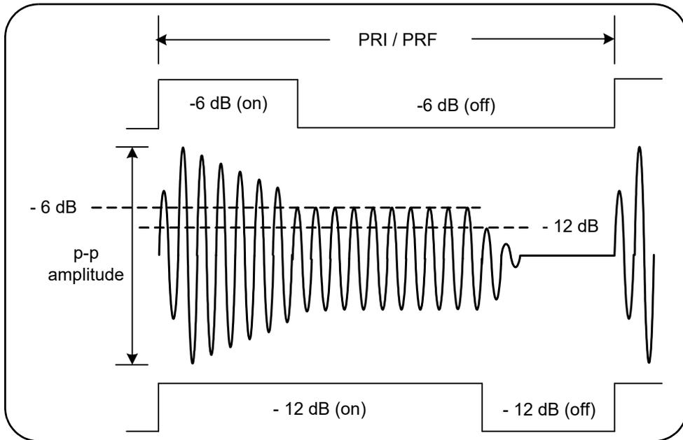
**Figure 4-6** -6 dB and -12 dB detector thresholds.
