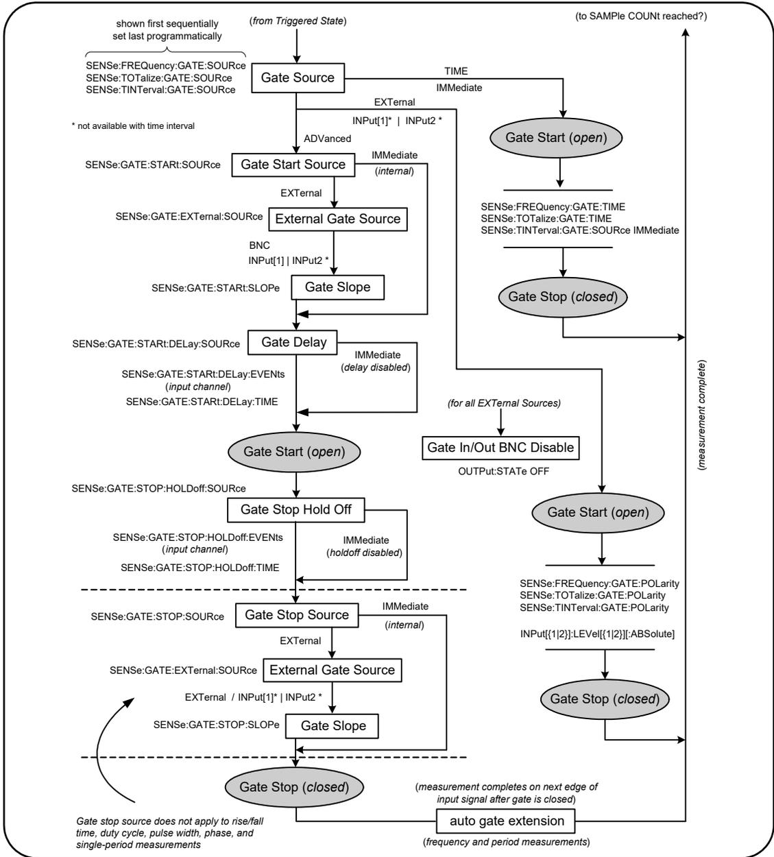
Figure 5-2 Trigger and gate cycle - gating (cont'd)
