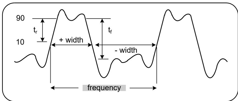
**Figure 3-2** Standard frequency measurement.
