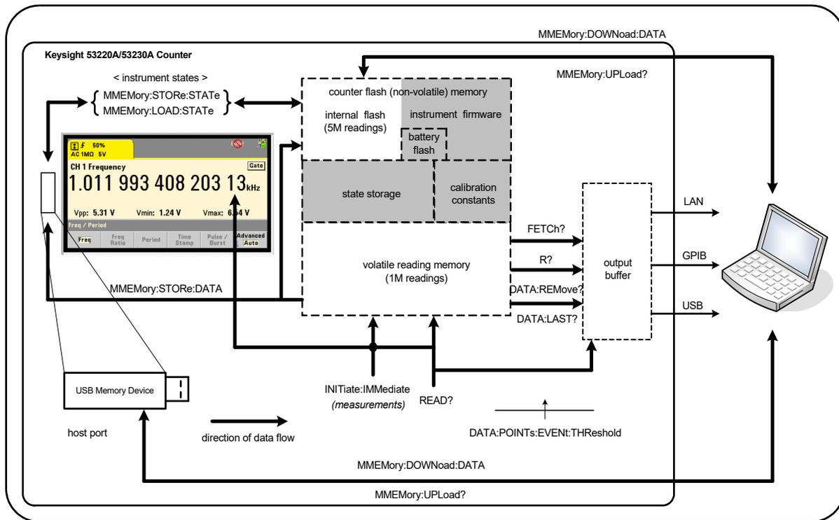
**Figure 7-1** Data flow within the 53220A/53230A counter.
