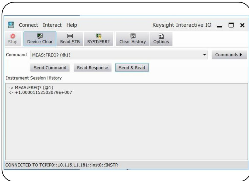
**Figure 2-2** The Web UI SCPI command interface.
