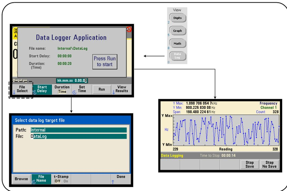
Figure 6-11 Starting the Counter Data Logger.
