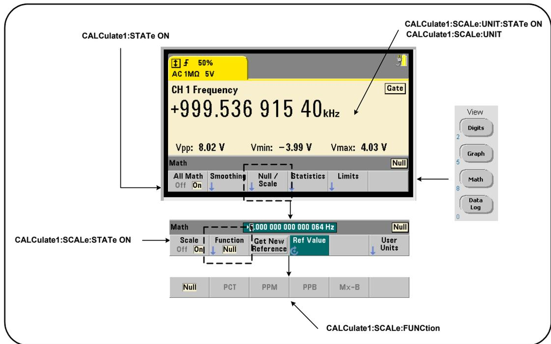
**Figure 6-2** 53220A/53230A display with scaling functions enabled.
