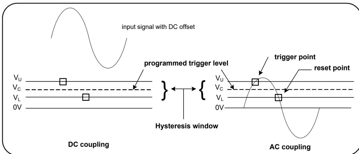
**Figure 4-2** Using AC coupling to reach trigger points.
