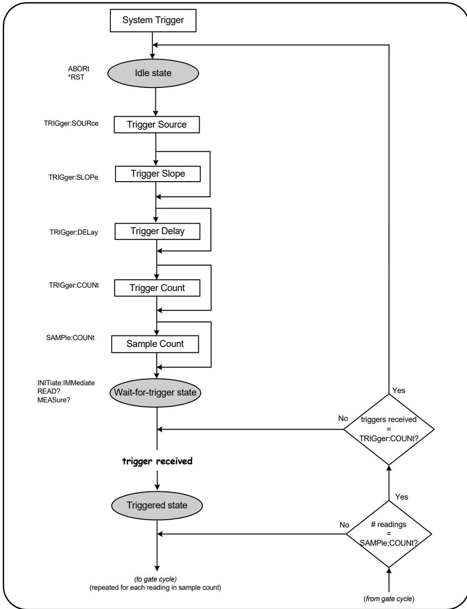
Figure 5-2 Trigger and gate cycle - triggering.
