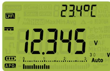
Figure 2-6 Filter for DC voltage measurements
