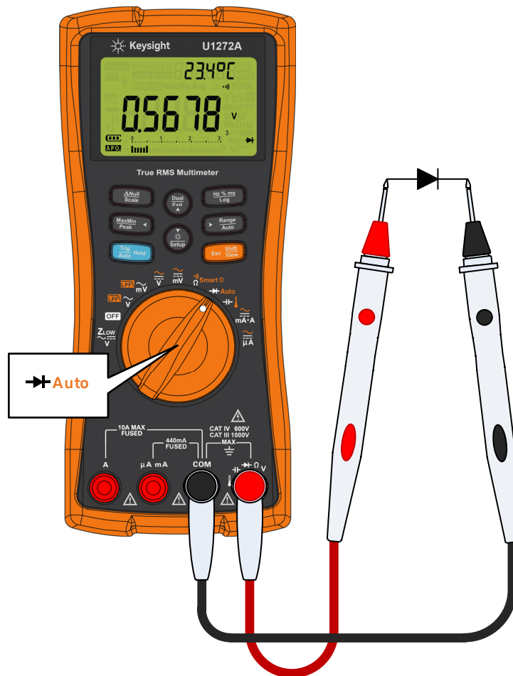
Figure 2-21 Testing forward bias diode
