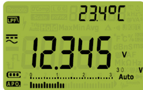
Figure 2-8 Low Pass Filter(LPF) for AC+DC voltage measurements
