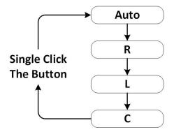
Figure 3-2: Switch Component Type by Single Clicking the Navigation Button
