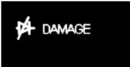
Figure 3-14: Display of Diode Measurement (Damaged Diode)
