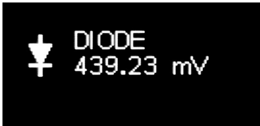
Figure 3-13: Display of Diode Measurement (Good Diode)
