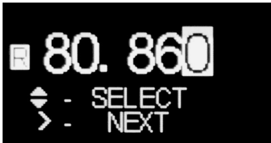
Figure 2-31: Input Digits of Reference Resistance Value
