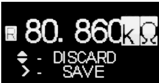
Figure 2-33: Save Reference Resistance Value from Inputting
