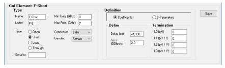
The coefficients L0 through L3 define the (parasitic) fringe inductance at the calibration point. Several Cal Kits have all these coefficients at zero.
