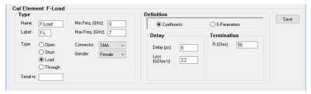
For the Load element the actual termination impedance can be specified.
