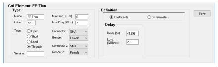
The Through element has no coefficients other than Delay and Loss.
