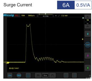
Surge current waveform at power adapter startup
