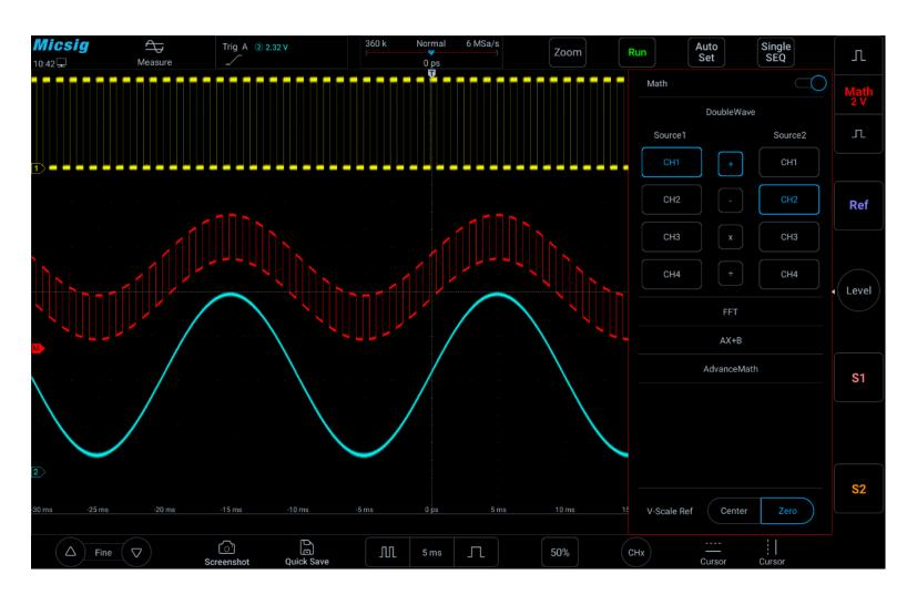
Figure 9-1 MATH Channel Waveform
