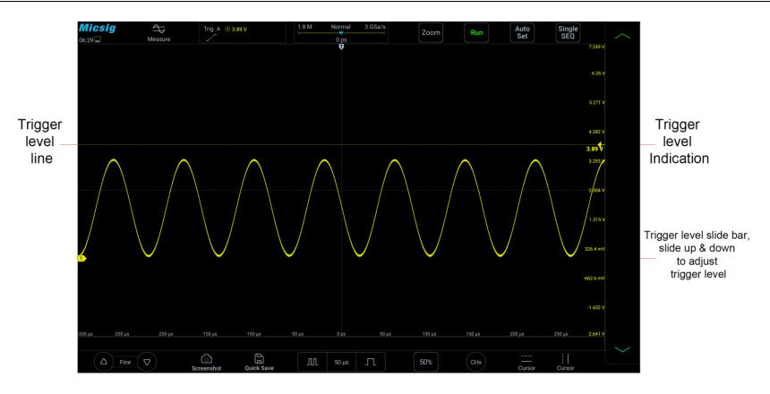
Figure 6-8 Trigger Level
