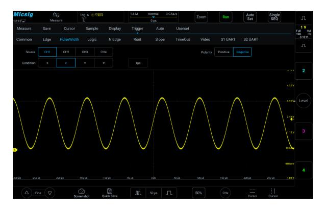
Figure 6-15 Negative Polarity Pulse Level Flip
