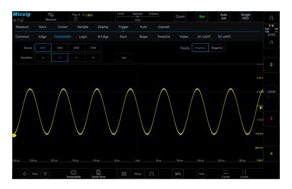
Figure 6-14 Pulse Width Trigger Setting Menu
