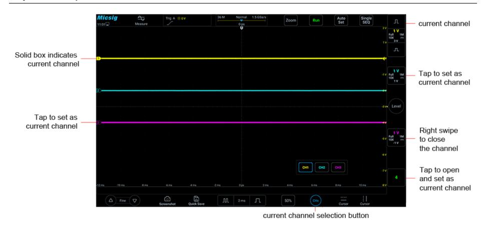
Figure 5-4 Channel Open, Close and Switching
