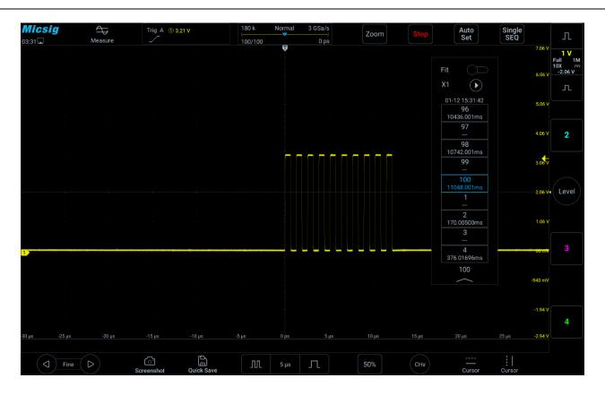
Figure 11-12 Segmented storage single frame viewing
