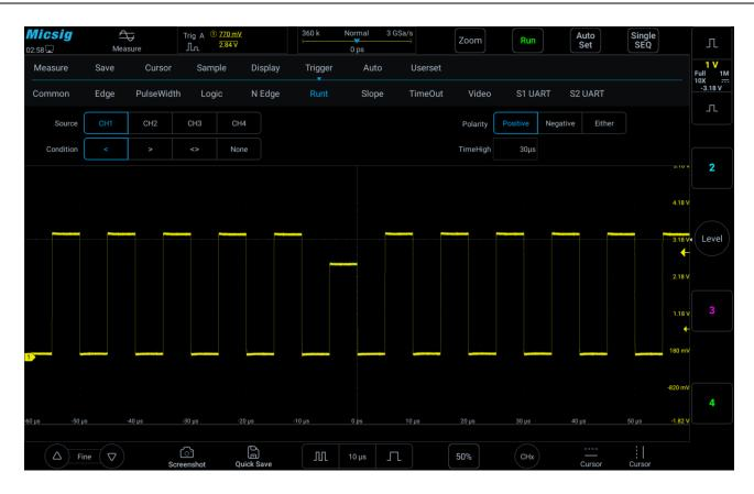
Figure 6-25 Runt Trigger Setting Menu
