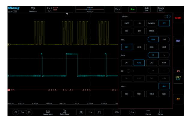
Figure 12-18 SPI Bus Configuration Menu
