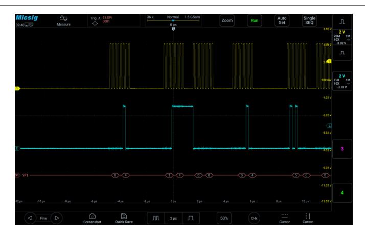
Figure 12-20 SPI bus decode interface
