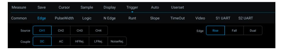
Figure 6-12 Edge Trigger Setting Menu
