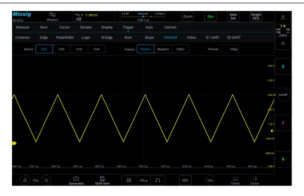
Figure 6-29 Time-out Trigger
