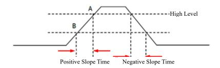
Figure 6-26 Positive/Negative Slope Time
