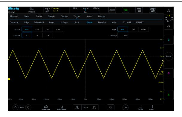
Figure 6-27 Slope Trigger Setting Menu
