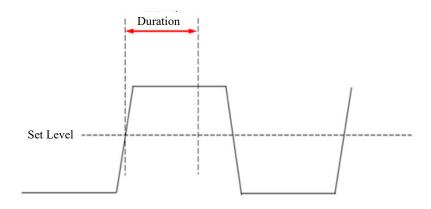
Figure 6-28 Timeout Trigger Schematics
