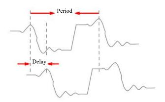
Figure 7-6 Phase Measurement Schematics
