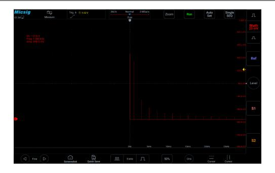
Figure 9-4 Spectrum Amplitude as V-Hz
