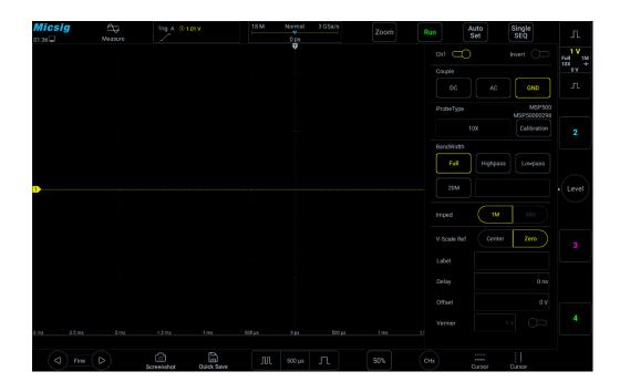
Figure 5-9 GND Coupling
