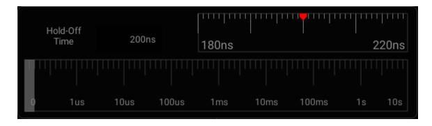
Figure 6-11 Trigger Hold-Off Time Set Interface
