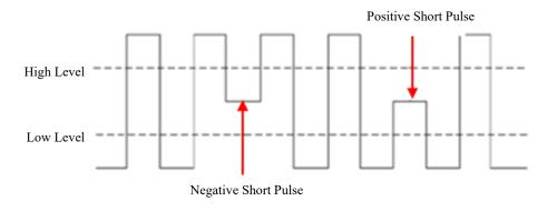
Figure 6-24 Runt Trigger
