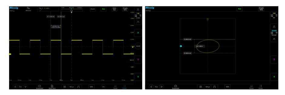
Figure 7-18 Cursor Measurement Pulse Width
