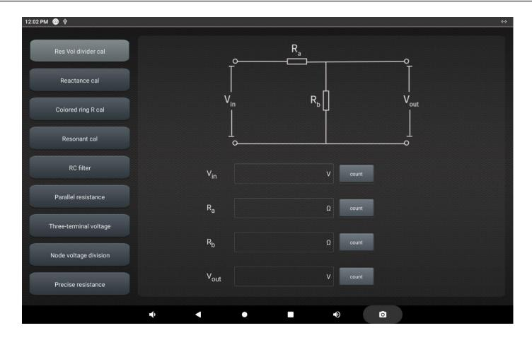
Figure 13-11 Electronic Calculation Tool Function
