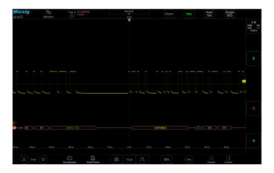
Figure 12-16 CAN bus decode interface
