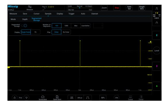
Figure 11-11 Segmented storage waveform acquisition
