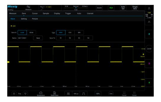
Figure 8-5 Save CH1 Reference Waveform Interface
