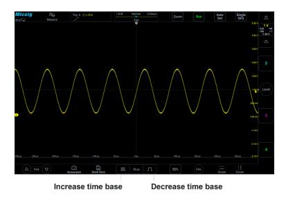
Figure 4-2 Adjust the Horizontal Time Base
