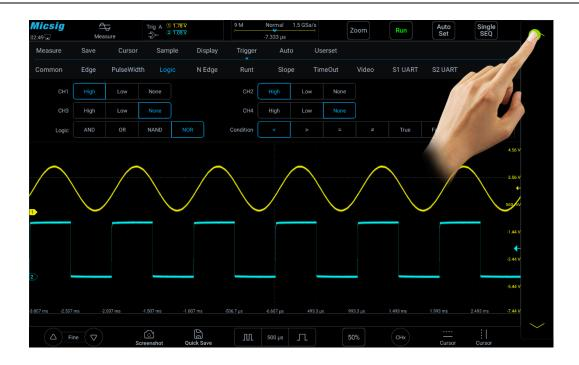
Figure 6-22 Trigger Level Adjustment
