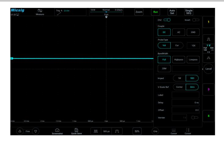
Figure 5-17 Channel input impedance
