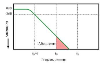
Figure 11-3 Sampling Rate and Oscilloscope Bandwidth
