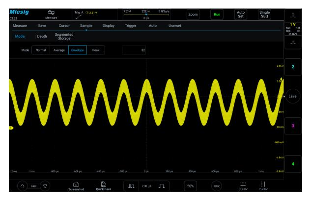
Figure 11-8 Signal in Envelope Sampling Mode (32)
