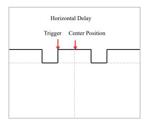
Figure 6-7 Horizontal Delay
