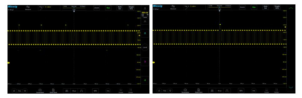
Figure 6-3 Abnormal Signal in Periodic Signals
