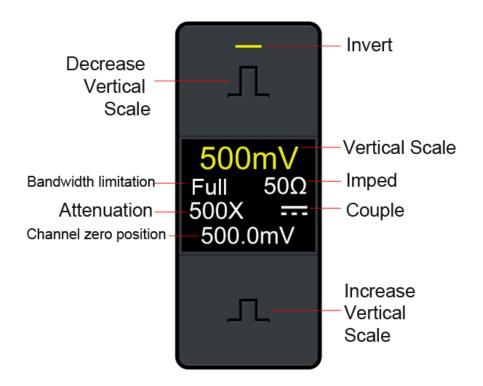
Figure 5-3 Channel Display Interface
