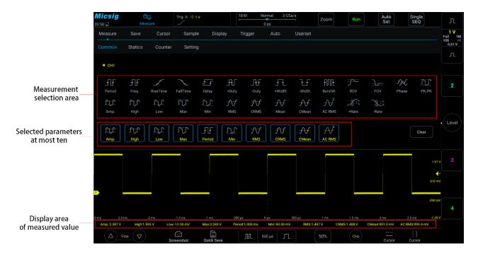
Figure 7-1 Automatic Measurement Menu
