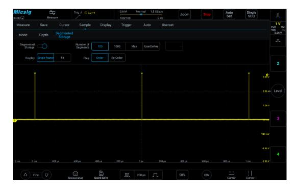
Figure 11-11 Segmented storage waveform acquisition
