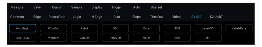
Figure 12-27 ARINC429 Trigger Mode Configuration Menu
