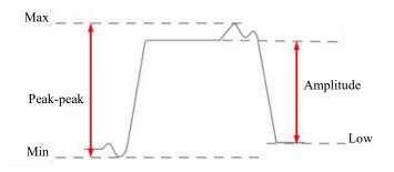
Figure 7-7 Voltage Measurement
