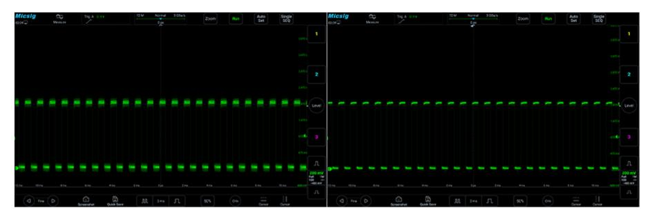
Figure 11-5 Sine Wave with Burr
