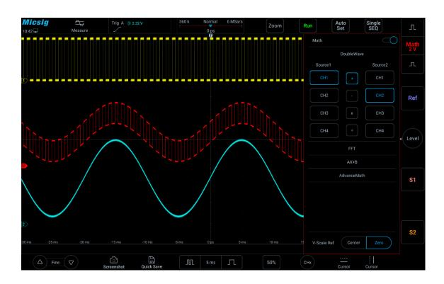
Figure 9-1 MATH Channel Waveform
