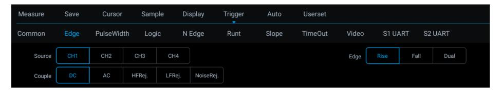
Figure 6-12 Edge Trigger Setting Menu
