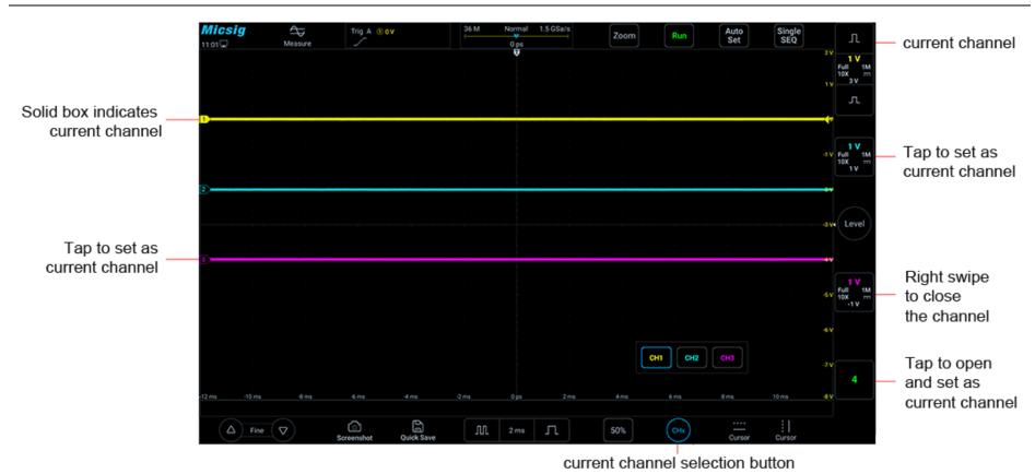
Figure 5-4 Channel Open, Close and Switching
