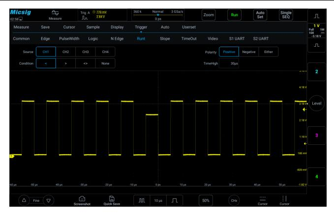
Figure 6-25 Runt Trigger Setting Menu
