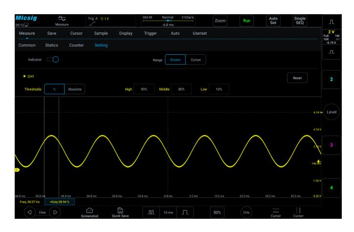
7-13 Pulse width when the median threshold value is set to 80%
