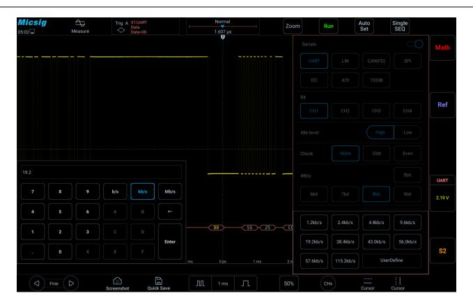
Figure 12-5 Baud Rate Default Setting
