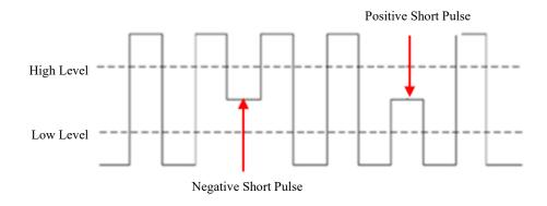
Figure 6-24 Runt Trigger
