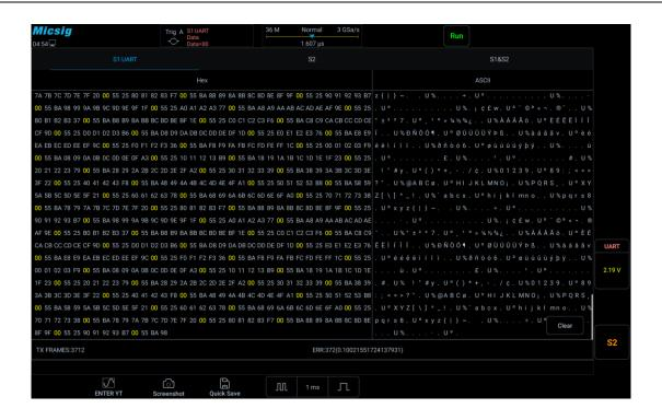
Figure 12-2 Bus Decode Text Mode
