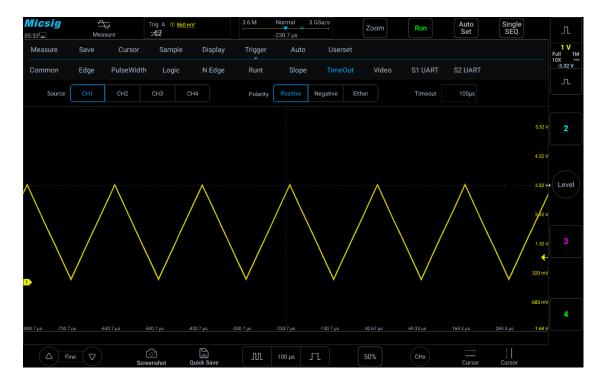
Figure 6-29 Time-out Trigger
