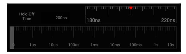
Figure 6-11 Trigger Hold-Off Time Set Interface
