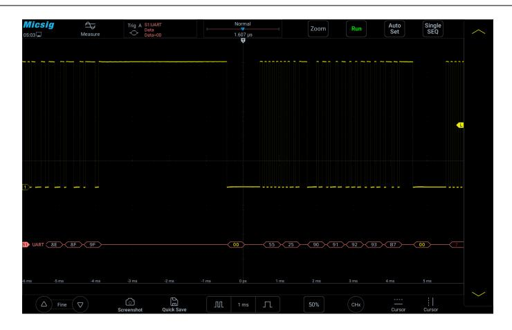
Figure 12-7 UART Decode Level Adjustment
