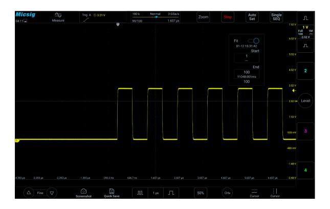
Figure 11-13 Segmented storage fitting view
