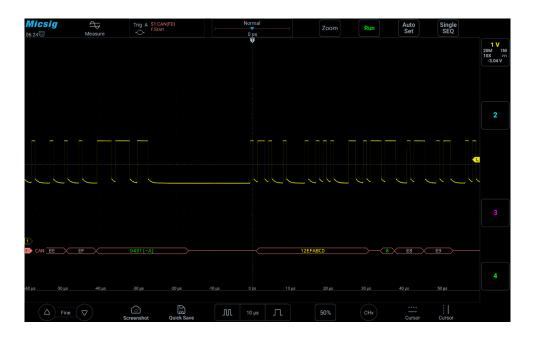
Figure 12-16 CAN bus decode interface
