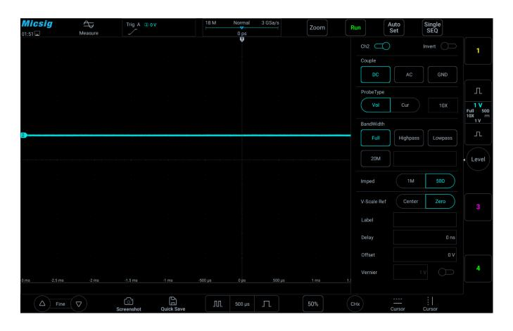
Figure 5-17 Channel input impedance
