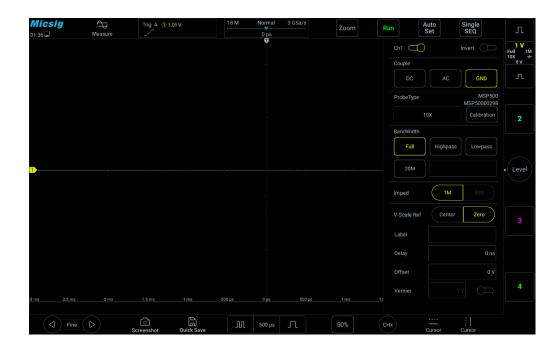
Figure 5-9 GND Coupling
