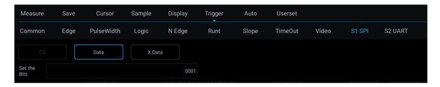
Figure 12-19 SPI Trigger Mode Configuration Menu
