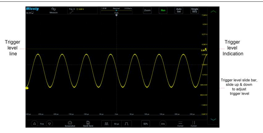
Figure 6-8 Trigger Level
