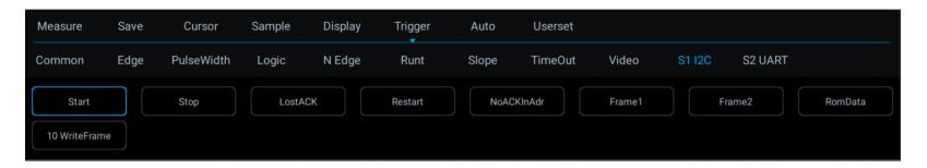
Figure 12-23 I<sup>2</sup>C Trigger Mode Configuration Menu
