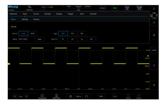
Figure 8-5 Save CH1 Reference Waveform Interface
