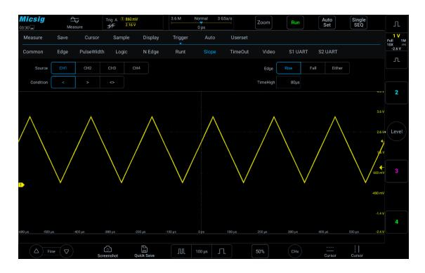
Figure 6-27 Slope Trigger Setting Menu
