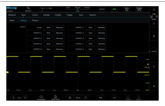
Figure 8-7 oscilloscope setting save
