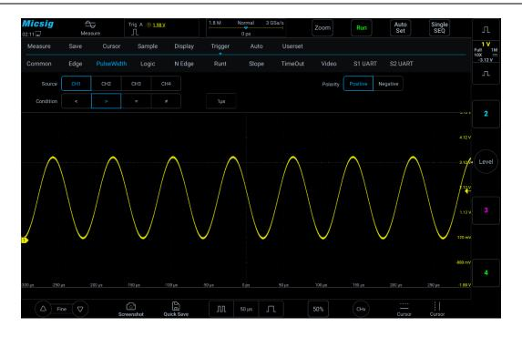
Figure 6-14 Pulse Width Trigger Setting Menu
