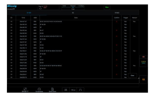
Figure 12-25 I<sup>2</sup>C Text Interface
