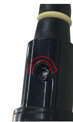
Use the trimmer to adjust the waveform.
