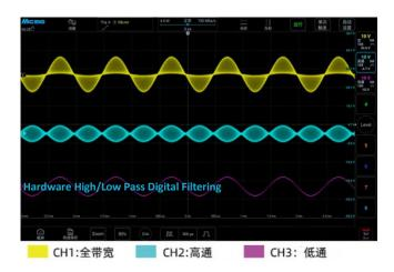
Hardware digital filtering effectively filters out interference and noise to improve signal accuracy and reliability. Digital filtering can selectively pass or block signal components in a specific frequency range.
