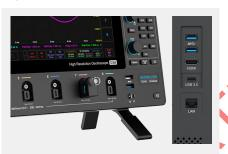
Unique Mic-OPI ™ probe interface, one-key automatic compensation; standard BNC adapter, can be adapted to any BNC interface probe. Equipped with USB 3.0/2.0 Host, USB Type-C, LAN, HDMI, Aux In/Out (support external trigger input, trigger output), 10MHz clock signal In/Out and other rich ports.
