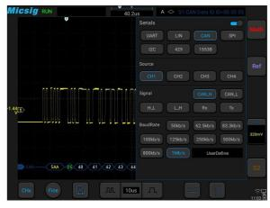
▲ Serial Bus Decoding and Analysis
