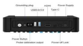
Complete connectivity (\* switch Power-off lock to ON for first-time use)
