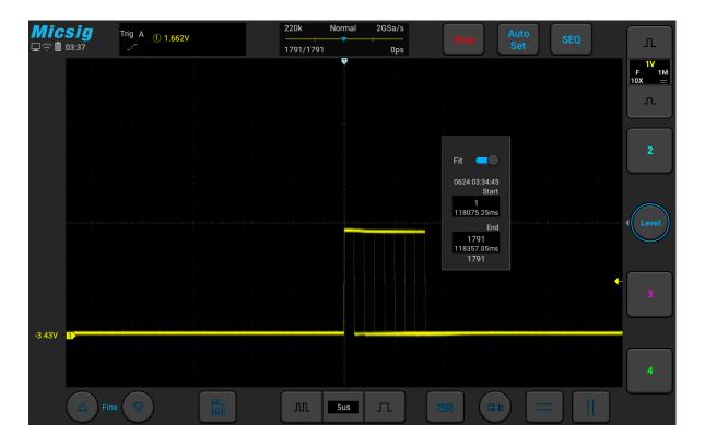
Figure 10-13 Segmented storage fitting view
