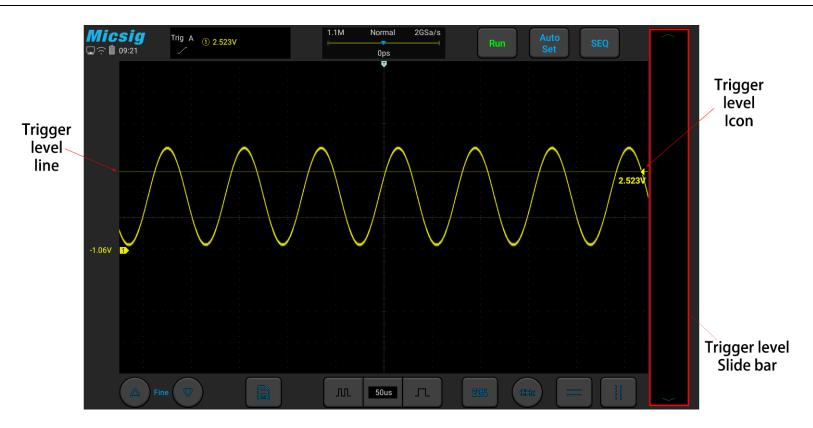
Figure 5-8 Trigger Level
