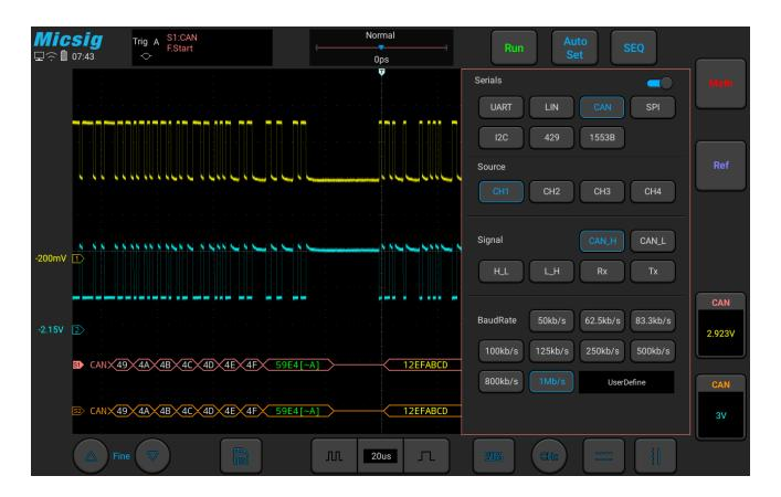
Figure 11-14 CAN Bus Configuration Menu
