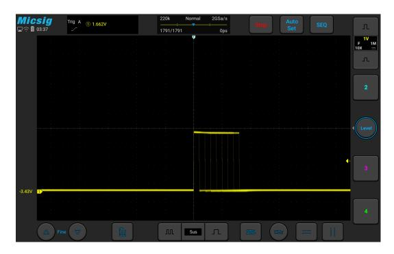
Figure 10-11 Segmented memory waveform acquisition
