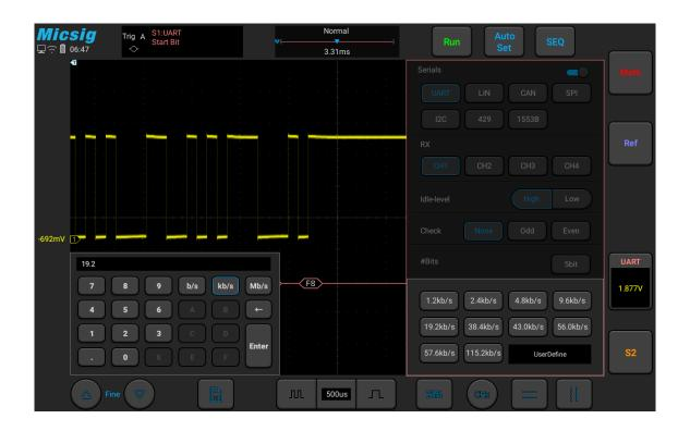
Figure 11-5 Baud Rate Default Setting
