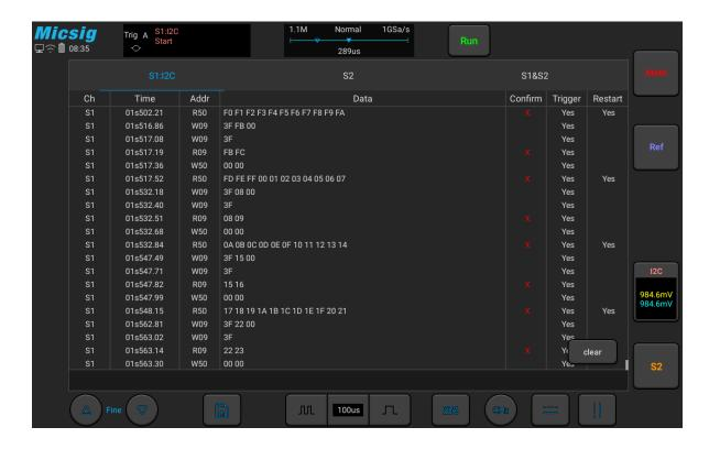
Figure 11-25 I2C Text Interface
