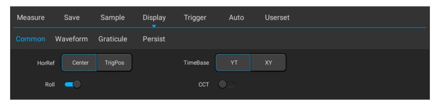
Figure 3-7 Roll Mode On/Off
