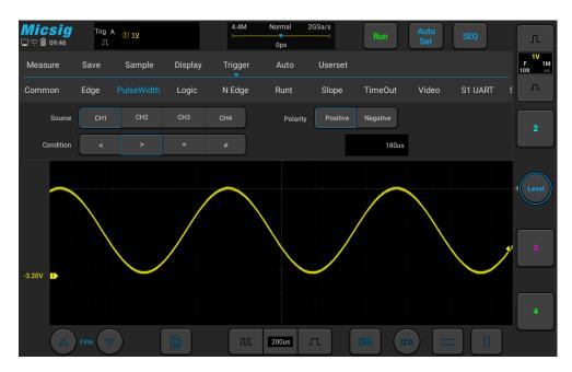
Figure 5-14 Pulse Width Trigger Setting Menu
