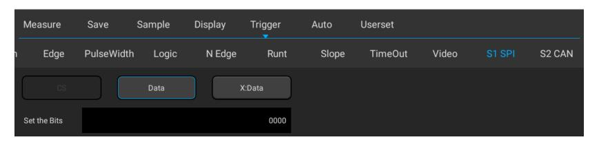
Figure 11-19 SPI Trigger Mode Configuration Menu
