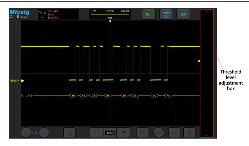
Figure 11-7 UART Decode Level Adjustment
