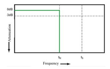
Figure 10-2 Theoretical Brick-Wall Frequency Response
