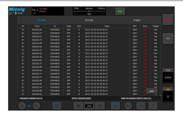
Figure 11-17 CAN Text Interface
