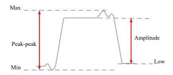
Figure 6-7 Voltage Measurement
