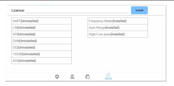
Figure 14-2 Decode Functions Not Installed
