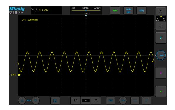
Figure 6-9 Frequency Meter Measurement
