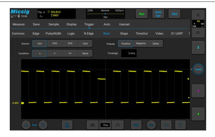
Figure 5-25 Runt Trigger Setting Menu
