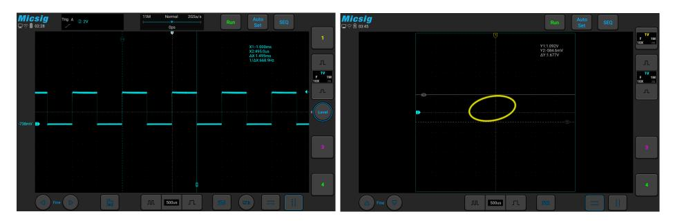
Figure 6-12 Cursor Measurement Pulse Width
