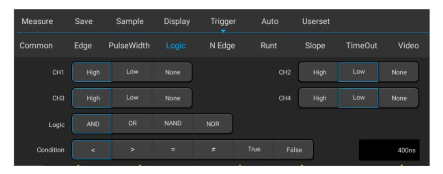
Figure 5-21 Logic Trigger Setting Menu
