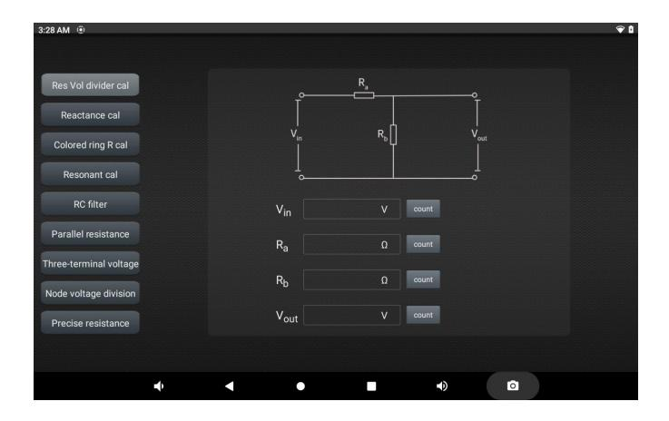
Figure 12-10 Electronic Calculation Tool Function
