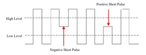
Figure 5-24 Runt Trigger
