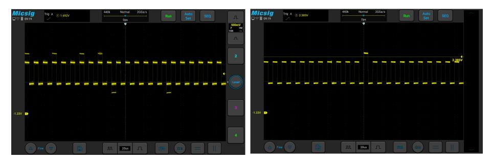
Figure 5-3 Abnormal Signal in Periodic Signals
