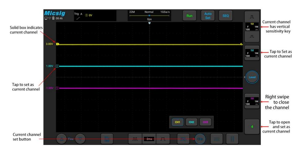
Figure 4-4 Channel Open, Close and Switching
