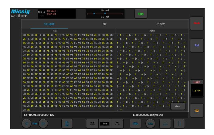
Figure 11-2 Bus Decode Text Mode
