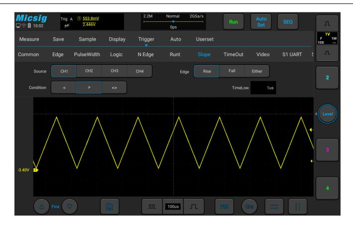
Figure 5-27 Slope Trigger Setting Menu
