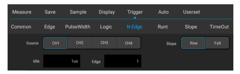
Figure 5-12 Edge Trigger Setting Menu
