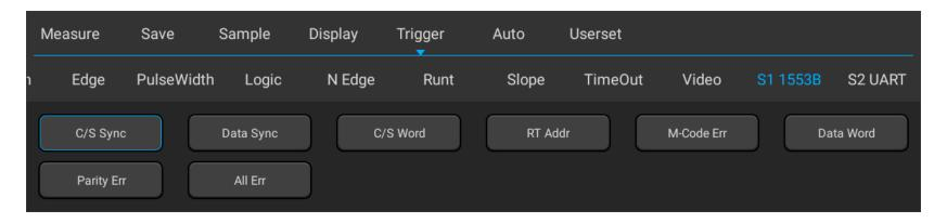
Figure 11-31 1553B Trigger Mode Configuration Menu
