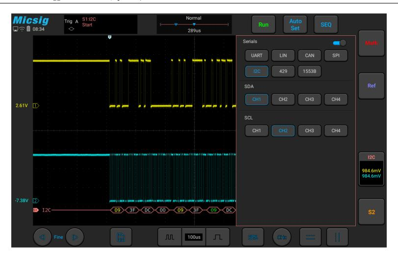
Figure 11-22 I2C Bus Configuration Menu
