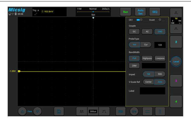
Figure 4-9 GND Coupling
