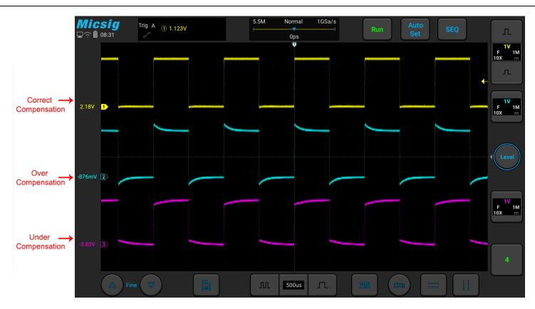
Figure 2-14 Probe Compensation
