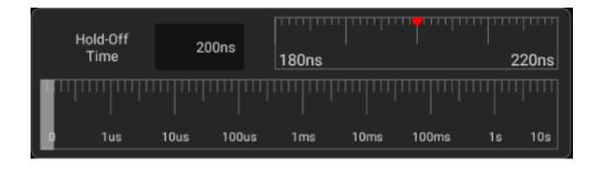
Figure 5-11 Trigger Hold-Off Time Set Interface
