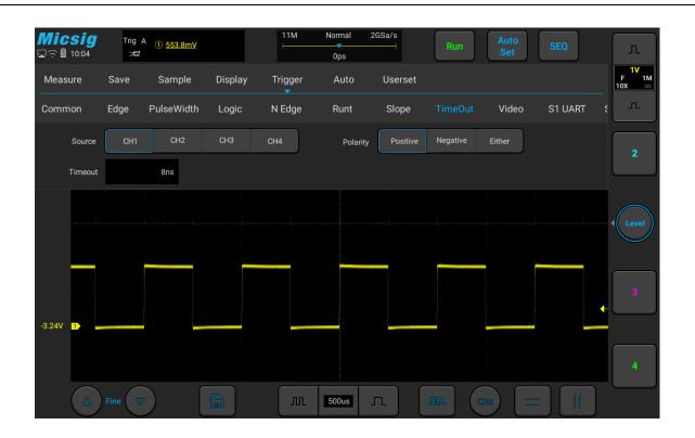
Figure 5-29 Time-out Trigger
