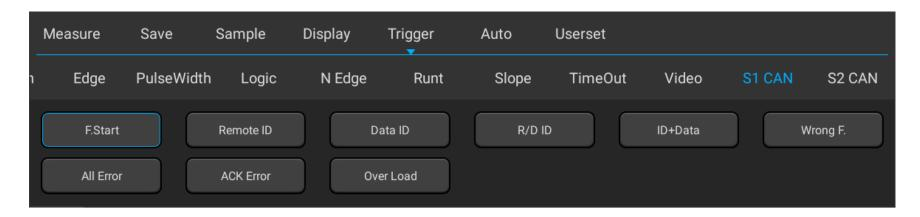
Figure 11-15 CAN Trigger Mode Configuration Menu
