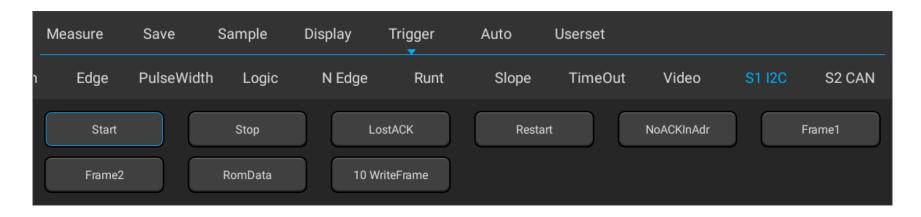
Figure 11-23 I2C Trigger Mode Configuration Menu
