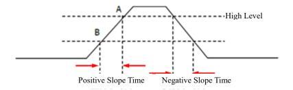
Figure 5-26 Positive/Negative Slope Time
