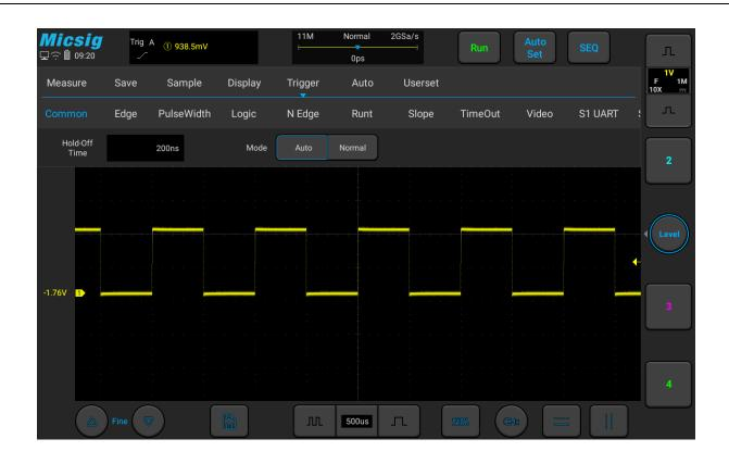
Figure 5-5 Oscilloscope Trigger Mode Setting
