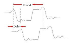
Figure 6-6 Phase Measurement Schematics
