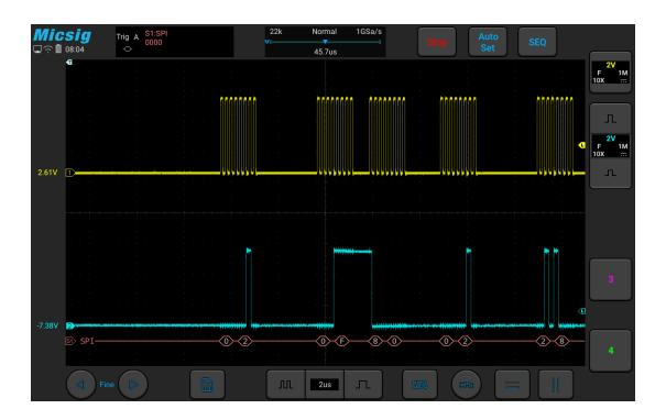
Figure 11-20 SPI Graphic Interface
