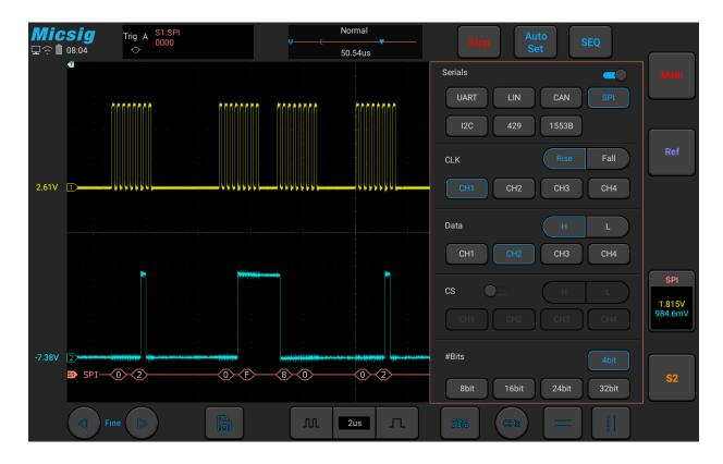
Figure 11-18 SPI Bus Configuration Menu
