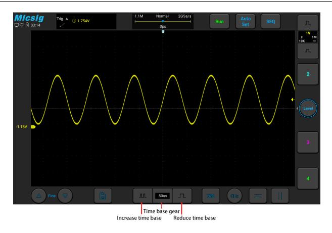
Figure 3-3 Adjust the Horizontal Time Base
