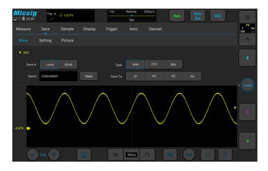
Figure 7-5 Save CH1 Reference Waveform Interface
