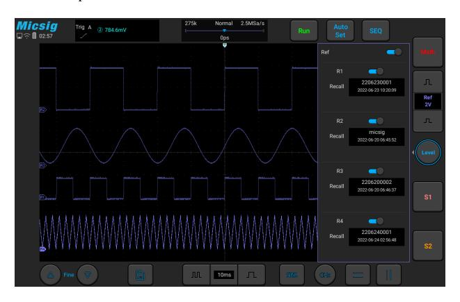
Figure 8-7 Restore Reference Waveform
