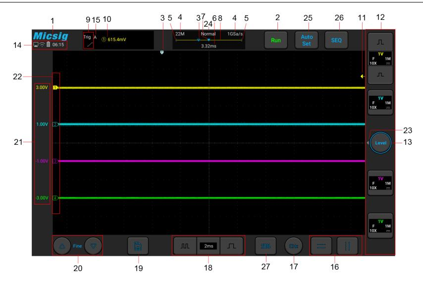
Figure 2-6 Oscilloscope Interface Display
