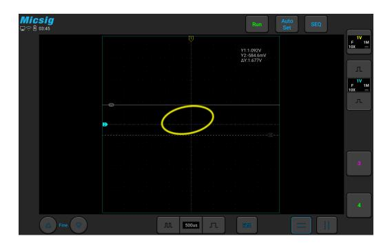
Figure 3-10 Phase Difference Measurement and Using the Cursor
