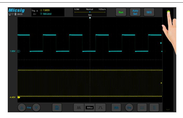
Figure 5-22 Trigger Level Adjustment
