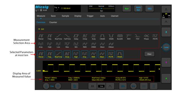
Figure 6-1 Automatic Measurement Menu
