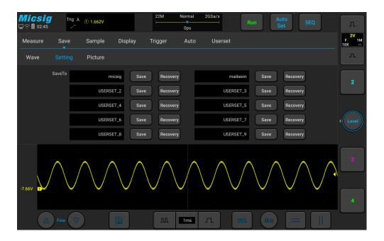
Figure 7-7 oscilloscope setting save
