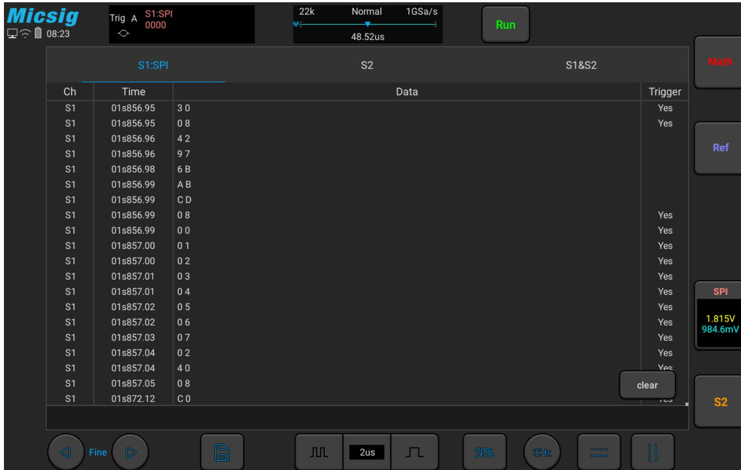
Figure 11-21 SPI Text Interface
