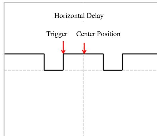
Figure 5-7 Horizontal Delay
