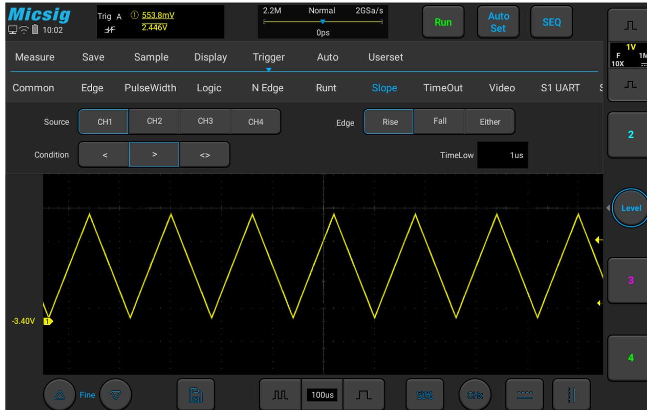
Figure 5-27 Slope Trigger Setting Menu
