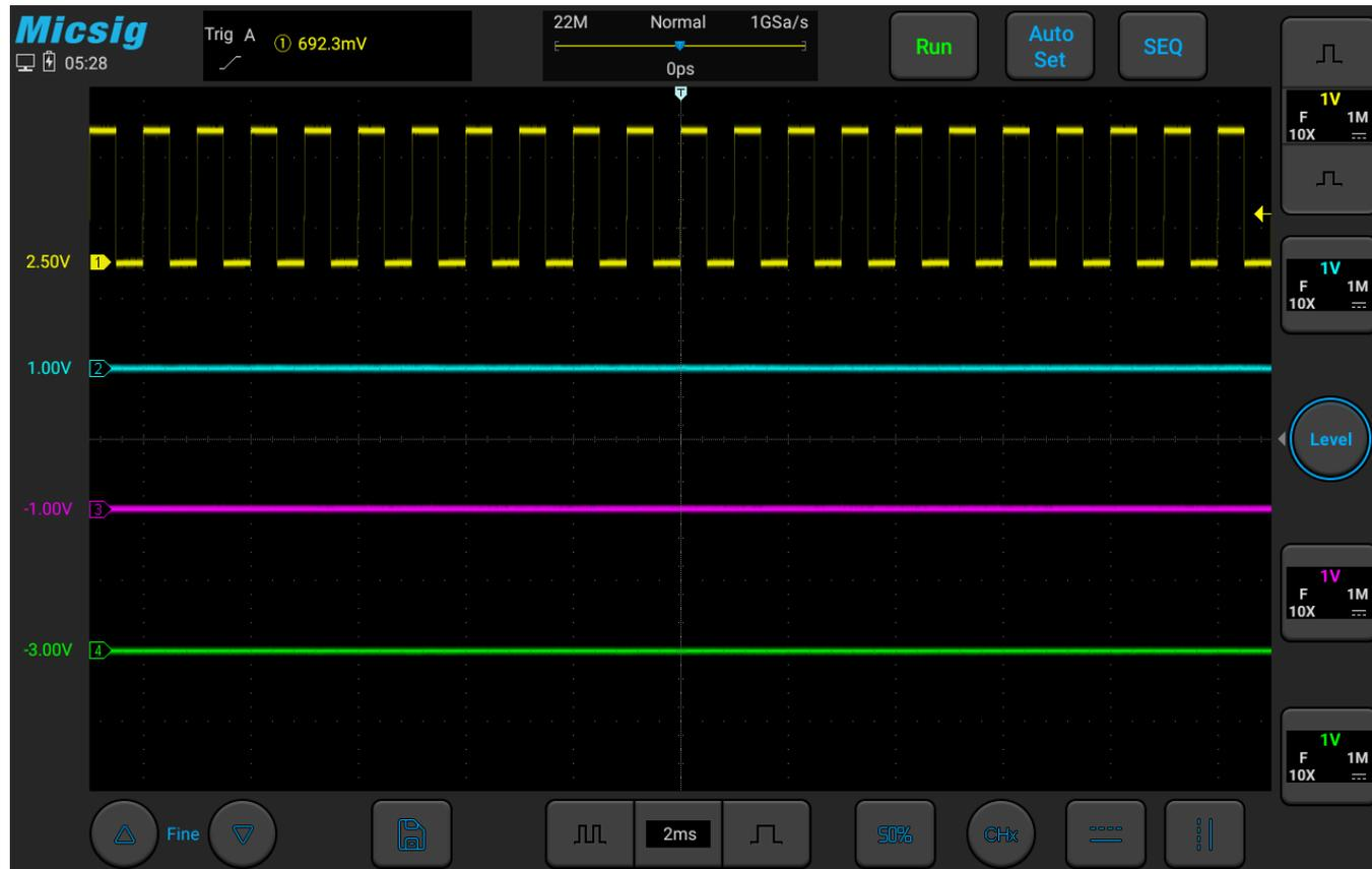
Figure 4-2 Current Channel and Non-Current Channel
