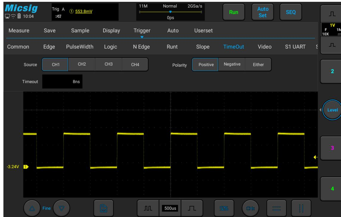
Figure 5-29 Time-out Trigger
