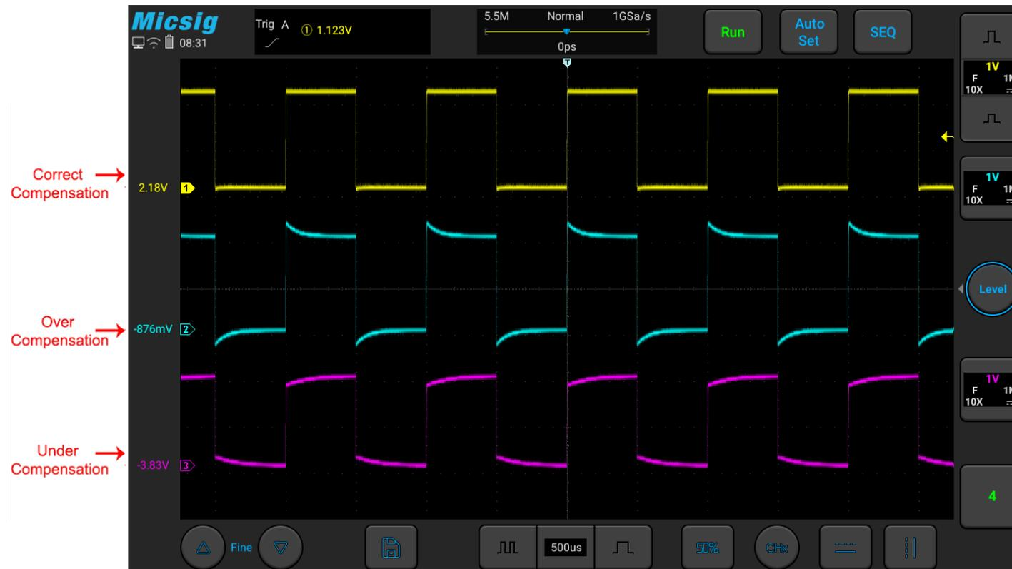
Figure 2-14 Probe Compensation
