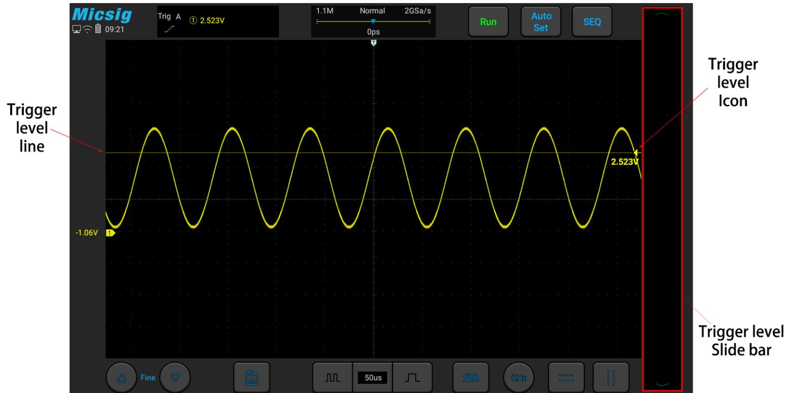
Figure 5-8 Trigger Level
