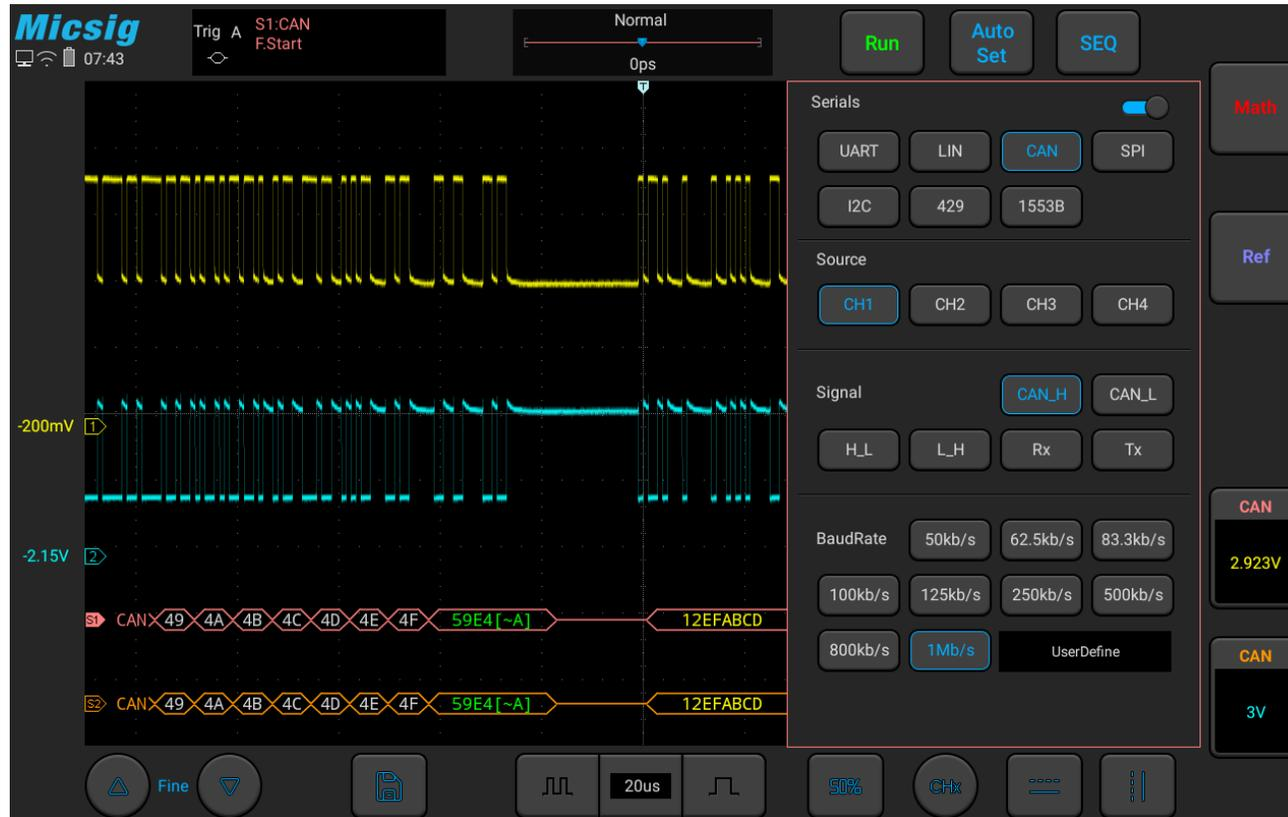
Figure 11-14 CAN Bus Configuration Menu
