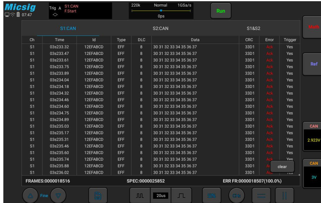
Figure 11-17 CAN Text Interface
