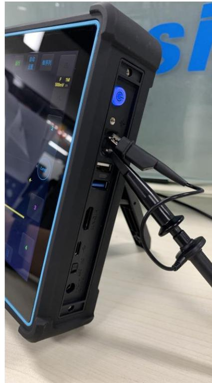
Figure 2-13 Probe Connection
