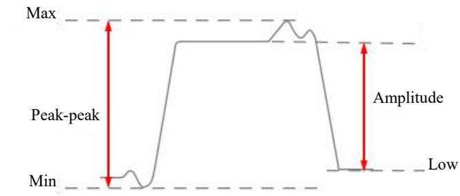
Figure 6-7 Voltage Measurement
