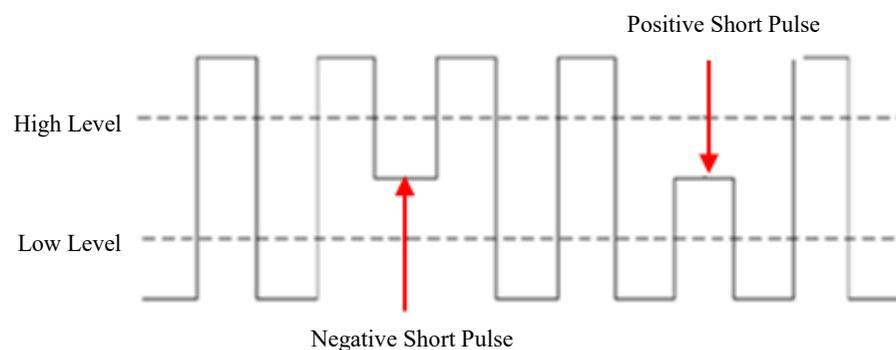
Figure 5-24 Runt Trigger
