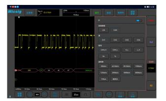
Bus decode Support CAN, LIN bus decoding.
