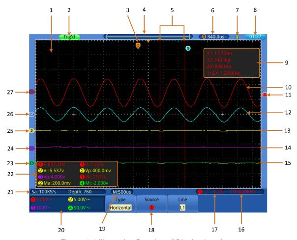
Figure 4-4 Illustrative Drawing of Display Interfaces
