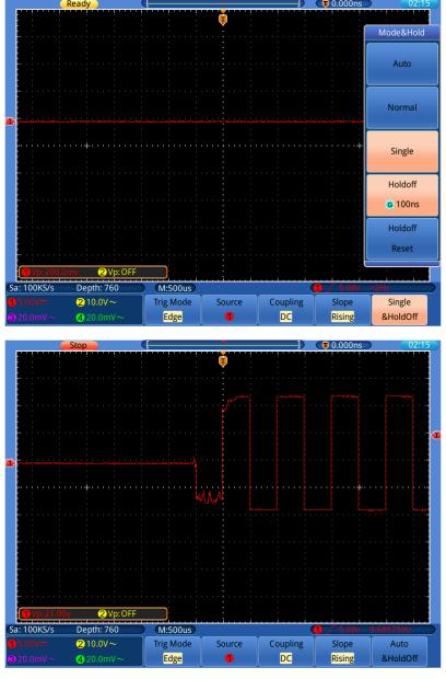
Figure 7-3 Capturing a Single Signal
