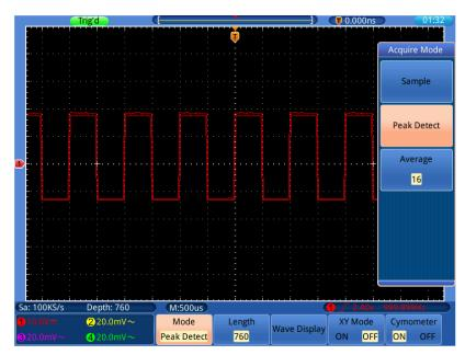
Figure 7-4 Signal with Noises
