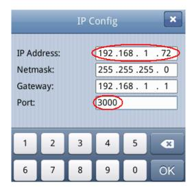
Figure 6-4 Set the network parameters of the oscilloscope
