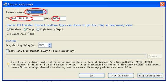
Figure 6-6 Set the network parameters of the Software
