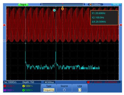
Figure 5-13 Wave of Freq cursor measurement
