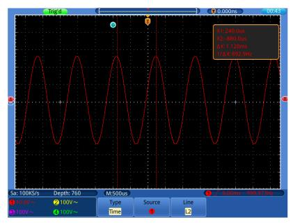
Figure 5-11 Waveform of Time Cursor Measurement
