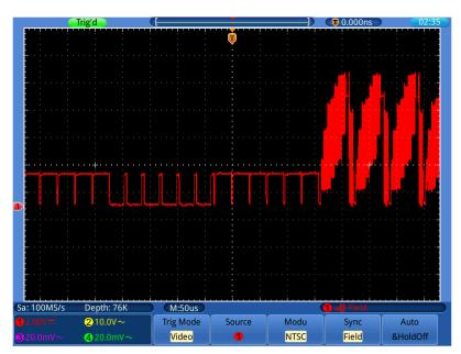
Figure 7-7 Waveform Captured from Video Field Trigger
