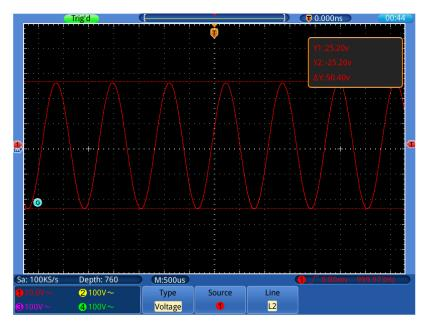
Figure 5-10 Waveform of Voltage Cursor Measurement
