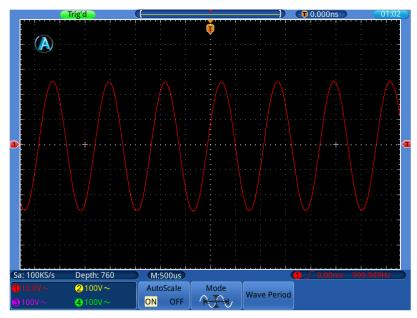
Figure 5-14 Autoscale Horizontal-Vertical multi-period waveforms
