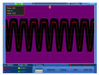
Figure 5-6 Pass/Fail test
