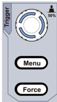
Figure 3-12 Trigger Control Zone
