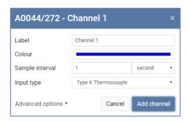
2. Click Add channel. The selected channel (in this case, channel 1) on the TC-08 will be highlighted in a color corresponding to the plot line Color chosen when the channel was set up. The Maths channel configurator will appear in the Devices tab as a small calculator. The thermocouple channel will be displayed in the Channels & Axes column on the right of the screen and also the Start recording, Pause, Delete, Save and Export buttons will be available:
