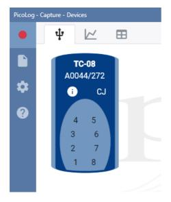
Select the channel corresponding to the location you chose for the thermocouple. The channel setup dialog will then display, allowing you to configure the channel. You can type in a channel Label and choose a channel Color, Sample interval and Input type (thermocouple type). You also have an advanced option to set Custom scaling:
