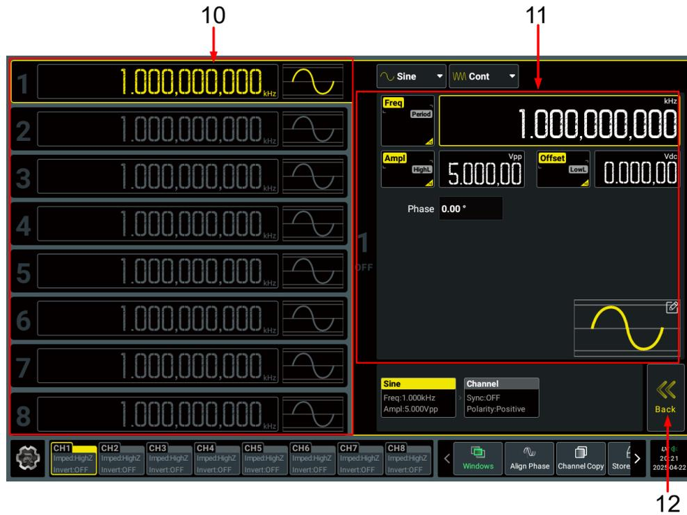
**Figure 4.15 8-Channel Display Mode Parameter Setting Interface**
