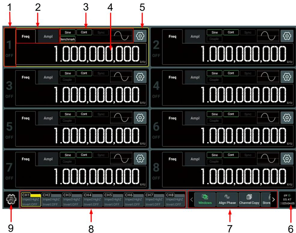
Figure 4.14 8-Channel Model User Interface - 8-Channel Display Mode
