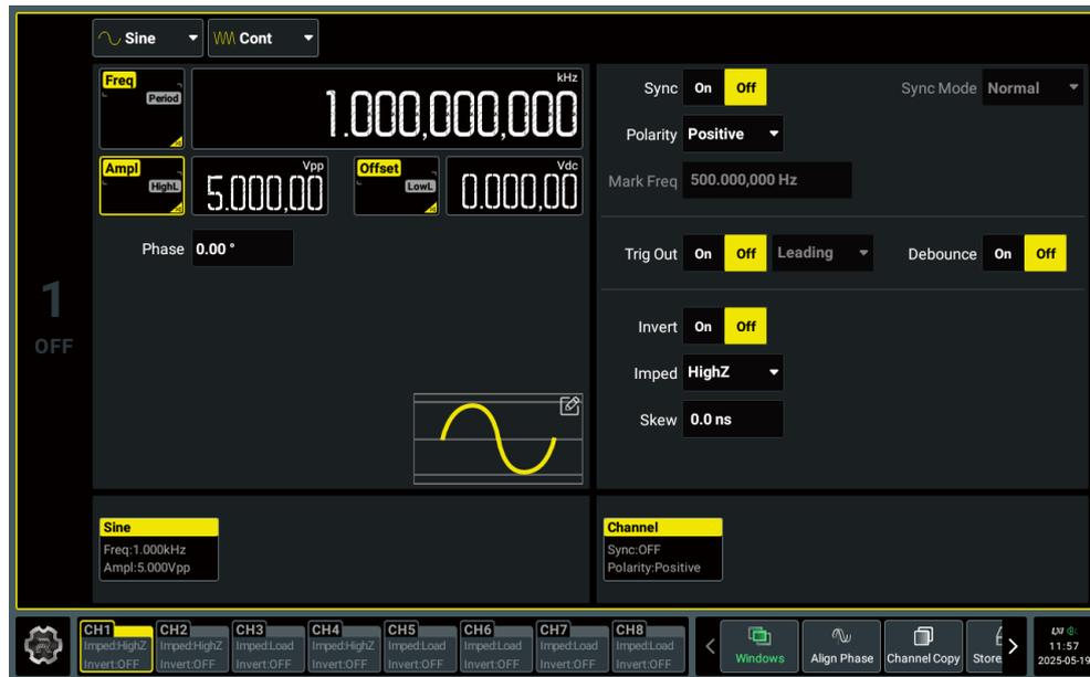
Figure 4.11 8-Channel Model User Interface - Single-Channel Display Mode
