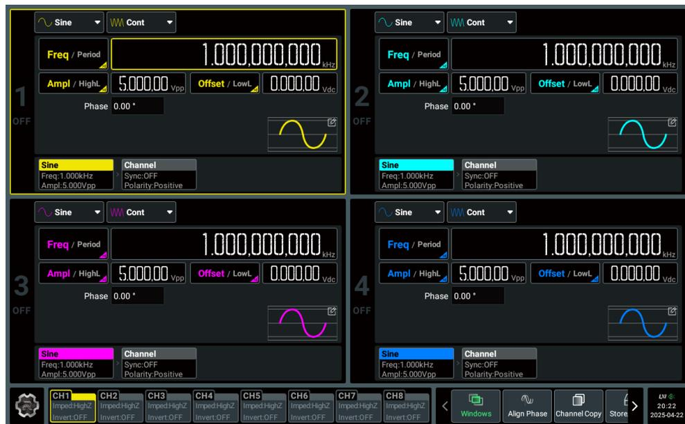
Figure 4.13 8-Channel Model User Interface - 4-Channel Display Mode
