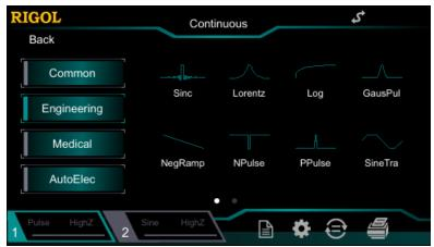
Figure 2-4 Arbitrary Waveform Selection Interface
