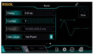
Figure 2-11 N Cycle Burst
