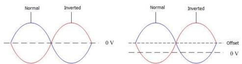
**Note:** When the waveform is inverted, the sync signal related to the waveform is not inverted. To set the invert of the sync signal, tap **SyncSet** → **Polarity** to select "Negative".
