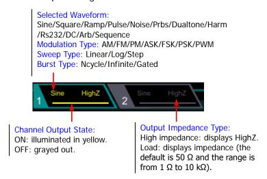
**Note:** Two channels can be enabled simultaneously, but you cannot select both channels at the same time.
