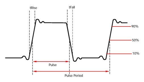
Tap the **RisEdge** or **FallEdge** parameter input field. Use the numeric keypad to input the desired value and then select the desired unit from the pop-up menu.
