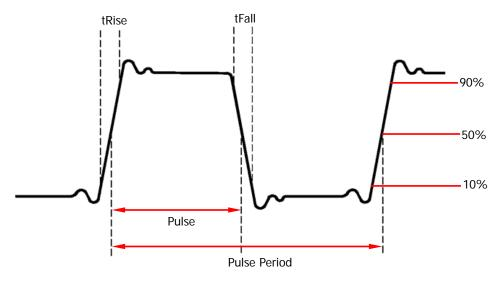
The settable range of the pulse width is from 16 ns to 999.999982118 ks (limited by "minimum pulse width" and "pulse period"). The default is 500 µs.
