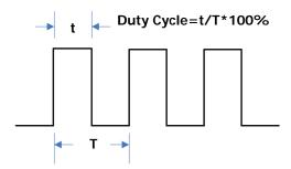
The available range of the duty cycle is from 0.01% to 99.99% (limited by the current frequency setting). The default is 50%.
