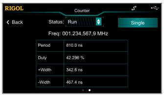
Figure 2-17 Frequency Counter Parameter Measurement Interface
