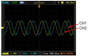
Figure 2-1 Before Aligning Phase
