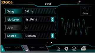
Figure 2-12 Infinite Burst
