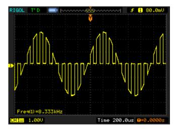
Figure 5-1 OSK Modulated Waveform
