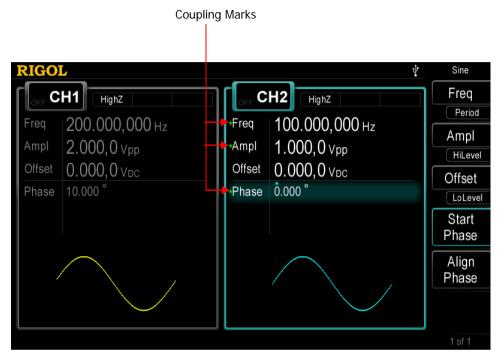
Figure 10-4 Channel Coupling
