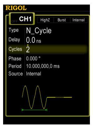
Figure 7-1 N Cycle Burst
