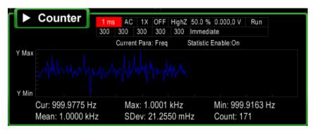
Figure 8-3 Curve Display Interface of the Statistic Results
