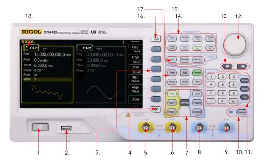
Figure 1-5 DG4000 Front Panel
