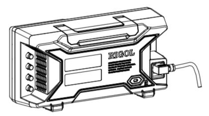
Figure 1-7 To Connect to Power
