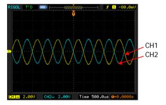
Figure 2-2 After Aligning Phase
