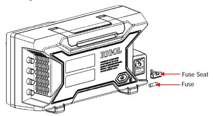
Figure 1-8 To Replace the Fuse
