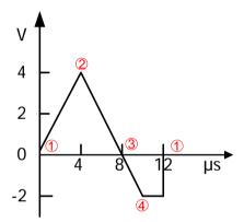
**Explanation:** As can be seen from the above figure, the waveform editor always connects the voltage levels of the first point to the last point in sequence and then hold this level until the cycle period expires to create a continuous waveform.
