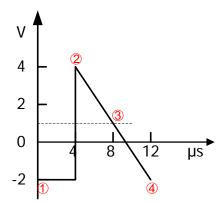
**Note:** As can be seen from the above figure, after the start point (point 2) and stop point (point 4) are inserted numerical values in the current interpolation method, the waveform editor will automatically generate point 1 and point 3 to create a continuous waveform.
