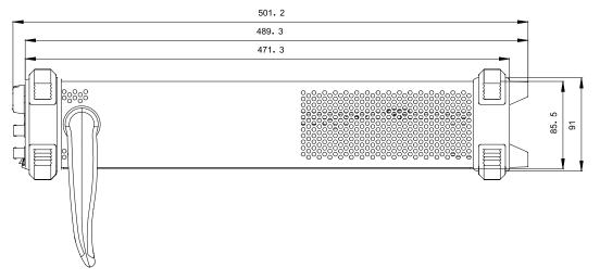
Side Elevation Unit: mm
