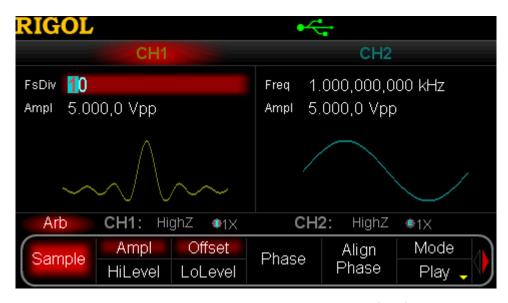
Figure 3-2 Arbitrary waveform output mode (Play)
