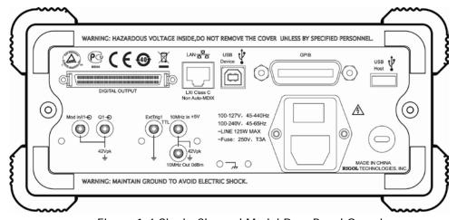
Figure 1-4 Single-Channel Model Rear Panel Overview
