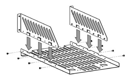
**3.** Place the instrument: align the protection pads of the instrument with the corresponding holes and then place it on the Support Board.
