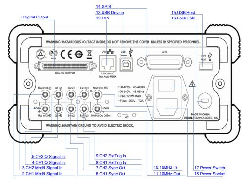
Figure 1-3 Dual-Channel Model Rear Panel Overview
