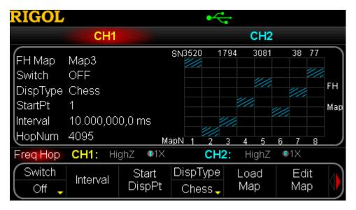
Figure 8-1 FH Function Setting Interface
