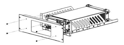
**6.** Load into the machine cabinet: mount the rack fixed with instrument into a standard 19-inch machine cabinet with four M6 screws and square nuts.
