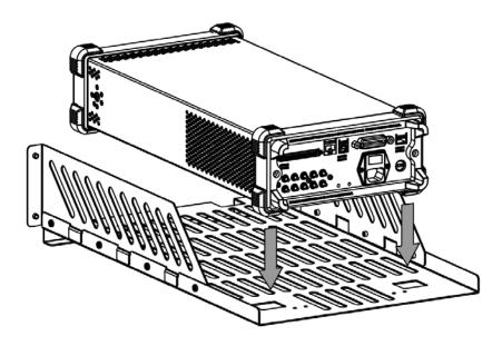
**4.** Fixed the instrument: Fasten the instrument tightly on the Support Board with two Fixed Figures and fixed it with four M4 screws.
