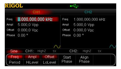
Figure 1-5 User Interface (Parameter Mode)
