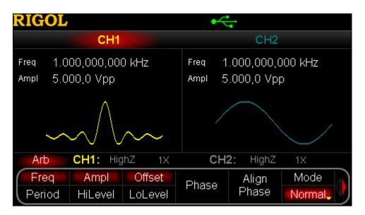
Figure 3-1 Arbitrary waveform output mode (Normal)
