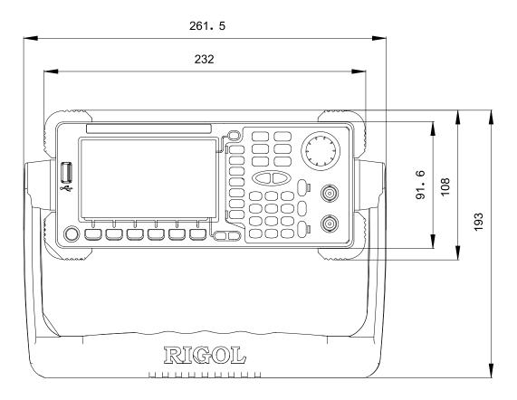
Front Elevation Unit: mm
