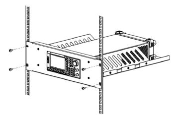
**7.** Post-installation notice: The rack occupies a height of 3U. The holes pointed out by the arrows are the installation holes. Note that they are aligned while installing.
