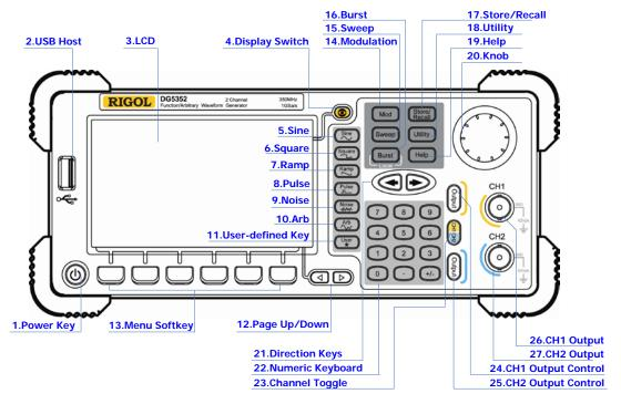
Figure 1-1 Dual-Channel Model Front Panel Overview
