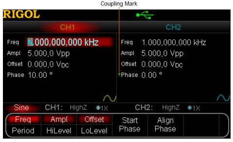
Figure 10-2 Channel Coupling
