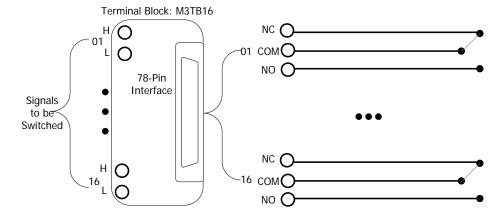
Figure 5-4 MC3416 Schematic Diagram
