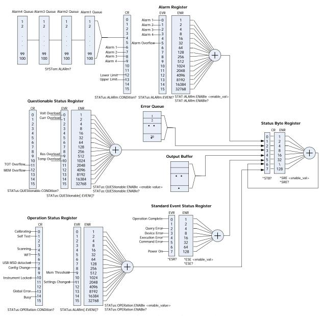
Figure 1-2 M300 Status System Structure Diagram
