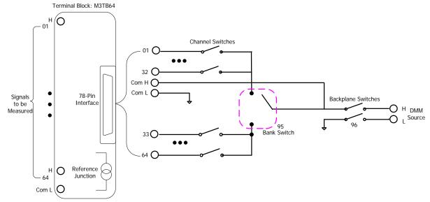
Figure 5-3 MC3164 Schematic Diagram
