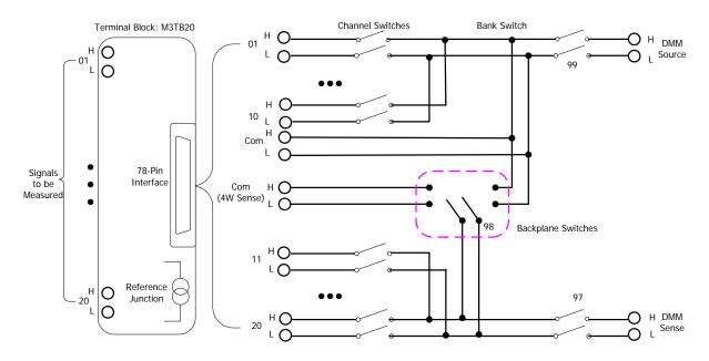
Figure 5-1 MC3120 Schematic Diagram
