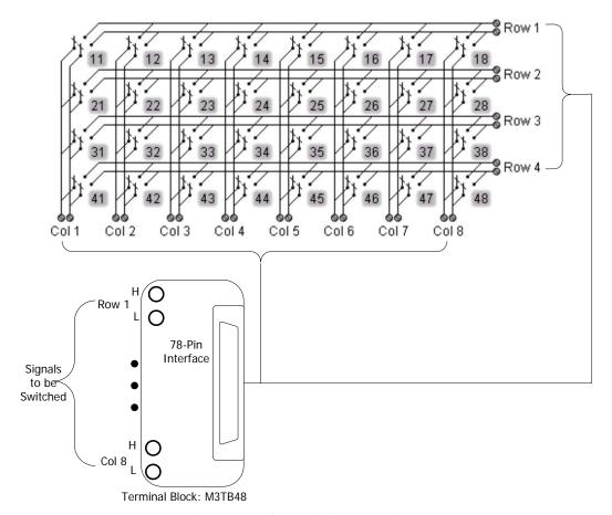
Figure 5-6 MC3648 Schematic Diagram
