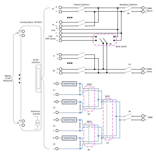
Figure 5-5 MC3324 Schematic Diagram
