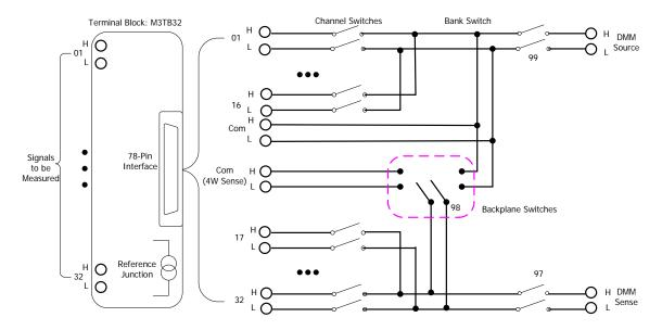
Figure 5-2 MC3132 Schematic Diagram
