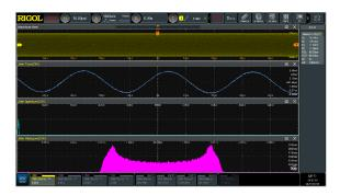
Perform TIE measurements on the clock signal with the jitter and analyze the results through the trend graph and histogram.
