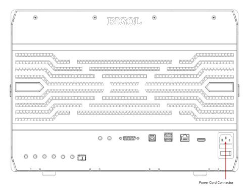
Figure 5.1 To Connect to AC Power
