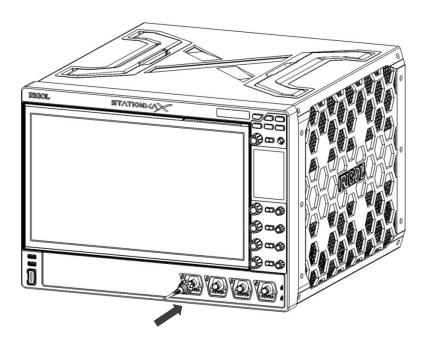
**Figure 5.2 To Connect the Passive Probe**
