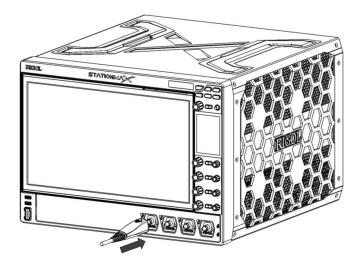
**Figure 5.4 To Connect the Active Probe**
