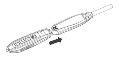
Figure 5.3 To Connect the Probe Head to the PA of the Active Probe
