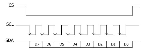
Figure 8.17 Sequential Chart of SPI Bus
