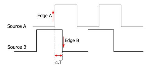
Figure 8.10 Delay Trigger
