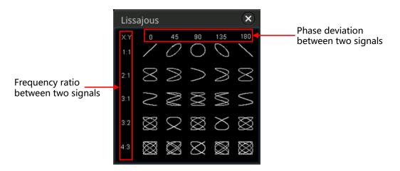
Figure 9.4 Lissajous Schematic Diagram
