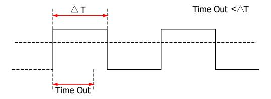
**Figure 8.8 Timeout Trigger**
