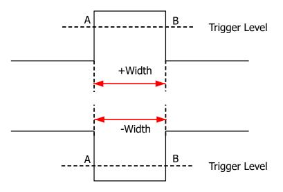
Figure 8.3 Positive Pulse Width/Negative Pulse Width
