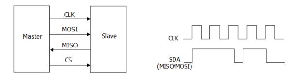
Figure 15.7 SPI Serial Bus
