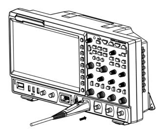
**Figure 4.8 Connect the Active Probe**
