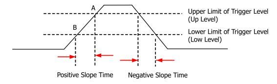
Figure 8.4 Positive Slope Time/Negative Slope Time
