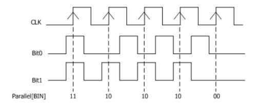
Figure 15.1 Schematic Diagram of Parallel Decoding
