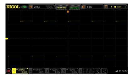
Figure 7.3 Waveforms after 128 Times of Averaging
