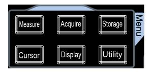
Press this key to enter the measurement setting menu. You can set the measurement source, enable or disable the all measurement function, the statistical analysis function, and etc. You can make a quick measurement for 41 waveform parameters.
