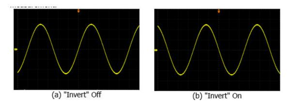
Figure 5.1 Waveform Invert
