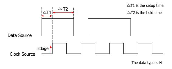
Figure 8.11 Setup/Hold Trigger
