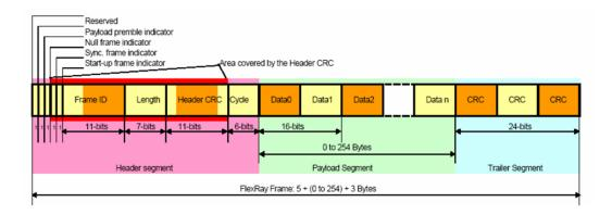
Figure 8.20 Frame Format of FlexRay Bus
