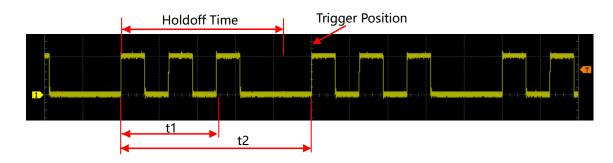
Figure 8.2 Schematic Diagram of Trigger Holdoff
