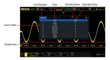
**Figure 15.2 Parallel Decoding Event Table**
