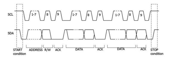
Figure 8.14 Schematic Diagram of I2C Protocol
