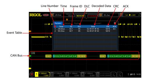
Figure 15.11 CAN Decoding Event Table
