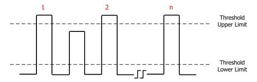
**2. Negative Pulse Count:** The number of negative pulses that fall from above the threshold upper limit to below the threshold lower limit.
