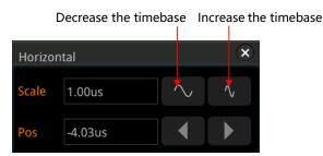
In the Horizontal control area (Horizontal) on the front panel, press the **Horizontal** SCALE knob to switch the adjustment mode between "Coarse" and "Fine" (by default, it is Coarse). You can also press More > Fine to enable or disable the fine adjustment of the horizontal time base.
