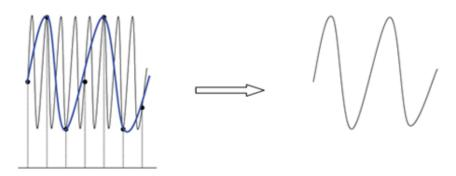
**3. Waveform Leakage:** when the sample rate is too low, the waveform rebuilt from the sample data do not reflect all the actual signal information.
