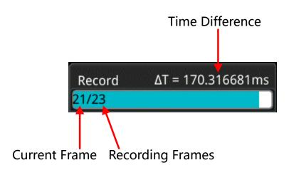
**Figure 18.1 Recording Process**
