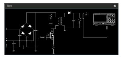
**Figure 11.2 Connection Diagram of Ripple Analysis**
