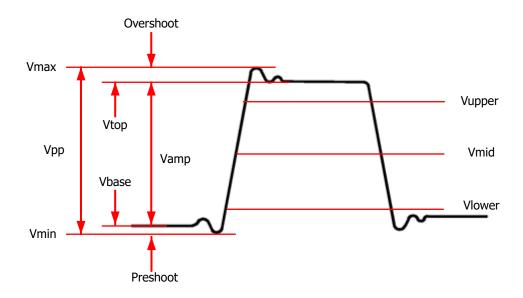
**Figure 9.2 Voltage Parameters**
