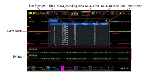
Figure 15.8 SPI Decoding Event Table
