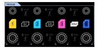
• 1, 2, 3, 4: indicates the analog channel switch key. The four channels are marked by different colors which are also used to mark both the corresponding
