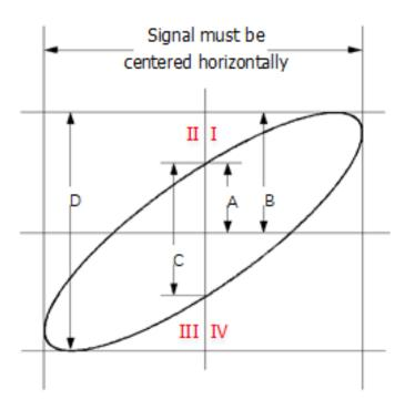
Figure 7.1 Measurement Schematic Diagram of Phase Deviation
