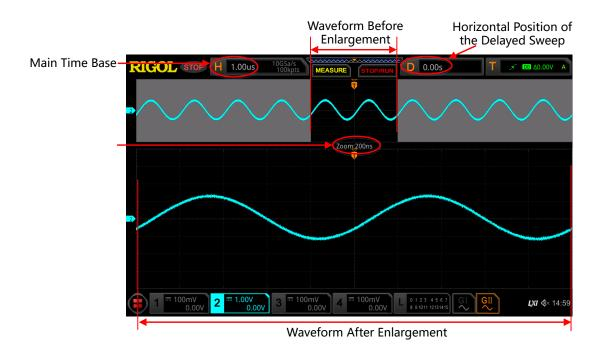
Figure 6.1 Delayed Sweep Mode
