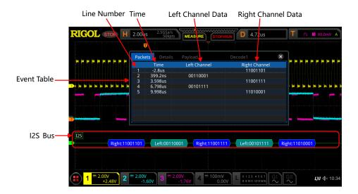
Figure 15.14 I2S Decoding Event Table
