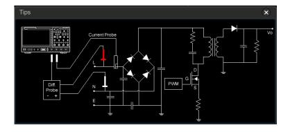
**Figure 11.1 Connection Diagram of Power Quality Analysis**
