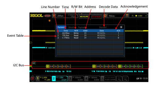
Figure 15.6 I2C Decoding Event Table
