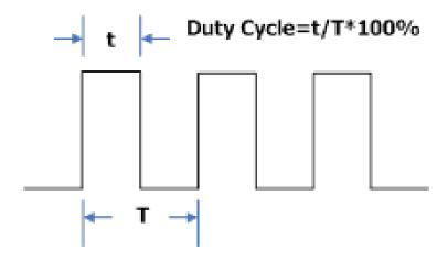
**Figure 21.2 Duty Cycle Definition**
