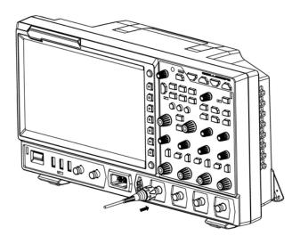
**Figure 4.6 Connect the Passive Probe**
