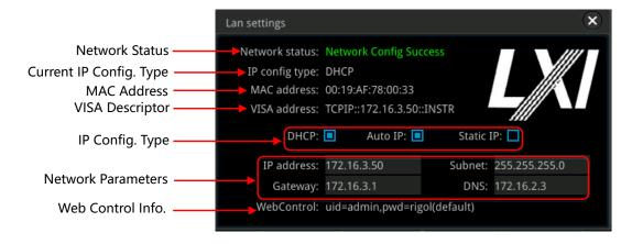
**Figure 23.1 Network Connection Setting Interface**
