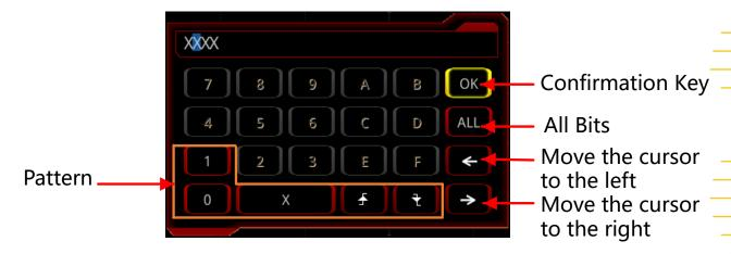
Figure 8.6 Virtual Keypad for Pattern Setting
