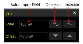
In the vertical control area (Vertical) on the front panel, press **Vertical** <u>SCALE</u> to adjust the vertical scale in "Coarse" (by default) or "Fine" mode. You can also press **More** > **Fine** to enable or disable the fine adjustment.
