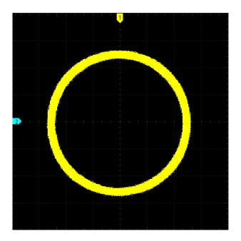
4. Observe the measurement result shown in the figure above. According to the measurement schematic diagram of the phase deviation (as shown in *Figure 7.1*),
