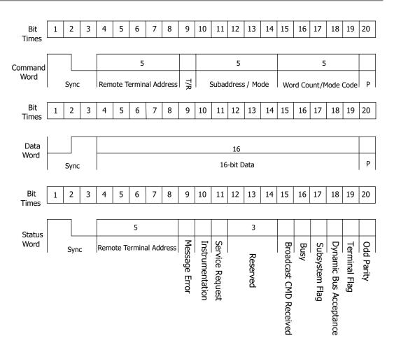
Figure 8.24 Formats of the Command Word, Data Word, and Status Word of the 1553B Bus
