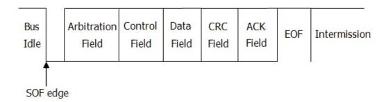
Figure 8.18 Data Frame Format of the CAN Bus
