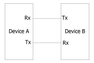
Figure 15.3 Schematic Diagram of RS232 Serial Bus
