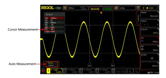
**Figure 9.3 Manual Cursor Measurement Example**
