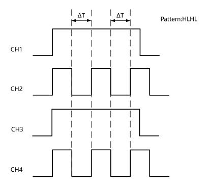
Figure 8.7 Duration Trigger
