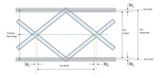
Figure 13.1 Diagram of Eye Measurement Parameters
