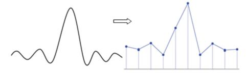
**2. Waveform Aliasing:** when the sample rate is twice lower than the actual signal frequency (Nyquist Frequency), the frequency of the waveform rebuilt from the sample data is smaller than the actual signal frequency.
