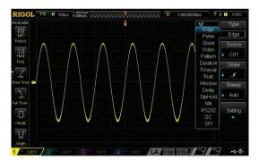
Built-in dual-channel 25 MHz source (DS1XX4Z-S Plus)
