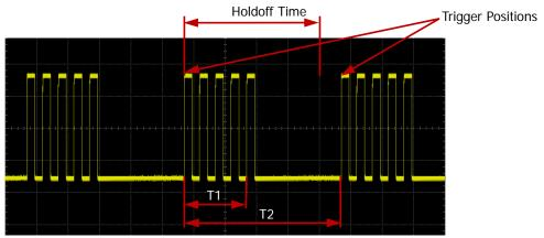
Figure 5-2 Schematic Diagram of Trigger Holdoff
