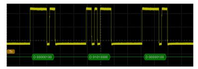
**Note:** Two error marks will be displayed when end frame error and check error are detected at the same time.
