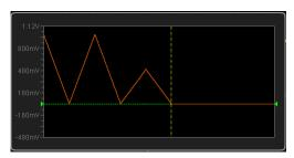
• **OFF:** the waveform editor will keep a constant voltage level between the two points and create a ladder-like waveform.
