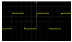
Figure 1-8 Probe Compensation Signal
