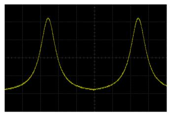
Figure 13-7 Lorentz Function Waveform
