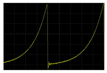
Figure 13-3 ExpRise Function Waveform
