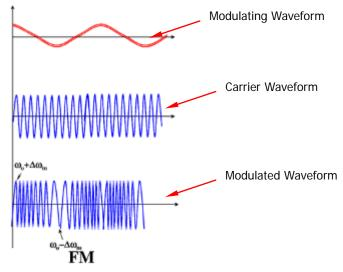
Figure 13-10 Frequency Modulation
