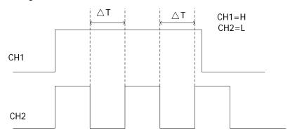
Figure 5-11 Duration Trigger
