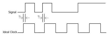
Figure 7-1 Digital Bus Jitter
