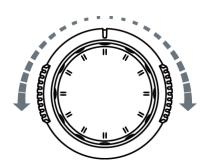
This knob can quickly adjust the numerical parameters with relatively large settable range. Turn clockwise (counterclockwise) to increase (reduce) the value. The inner knob is used for fine adjustment and the outer knob for coarse adjustment.
