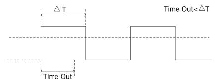
Figure 5-10 TimeOut Trigger
