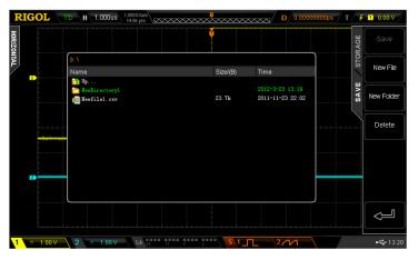
Figure 14-4 External Disk (To Select the Storage Position)
