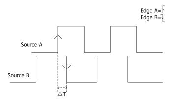
Figure 5-9 Delay Trigger
