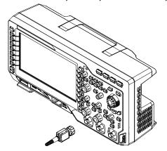
Figure 1-5 To Connect the Passive Probe
