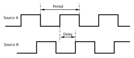
Figure 6-4 Delay and Phase
