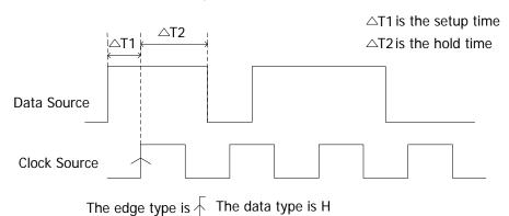
Figure 5-12 Setup/Hold Trigger
