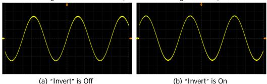
Figure 2-1 Waveform Invert
