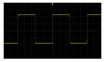
Figure 4-2 The Waveform after 256 Averages
