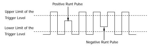
Figure 5-4 Runt Trigger
