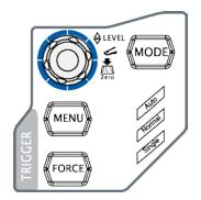
**MODE**: press this key to switch the trigger mode to **Auto**, **Normal** or **Single** and the corresponding state backlight of the current trigger mode would be illuminated
