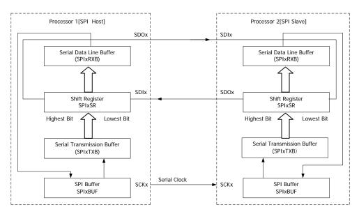
Figure 5-15 SPI Trigger
