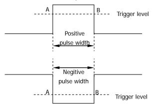
Figure 5-3 Positive Pulse Width/Negative Pulse Width
