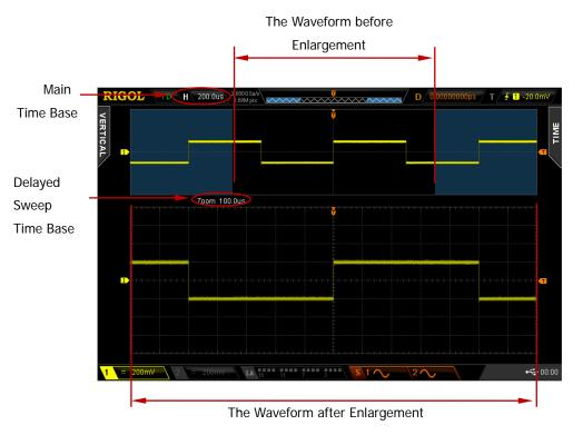
Figure 3-1 Delayed Sweep
