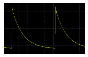
Figure 13-4 ExpFall Function Waveform
