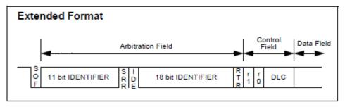
Figure 5-17 Standard and Expanded Formats of CAN Bus Data Frame
