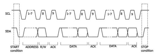
Figure 5-14 I2C Trigger
