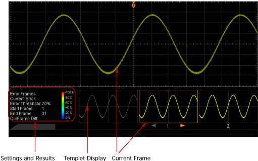
Figure 11-3 Waveform Analysis
