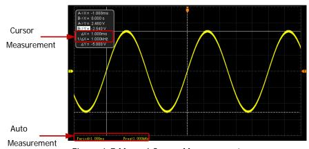
Figure 6-7 Manual Cursor Measurement
