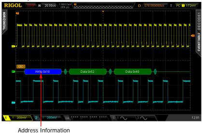
Figure 8-8 Address Information during Decoding
