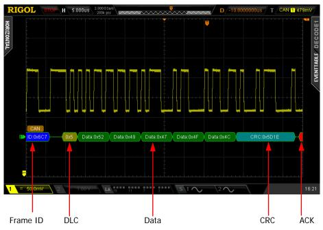
Figure 8-15 Decoded CAN Data Interpretation
