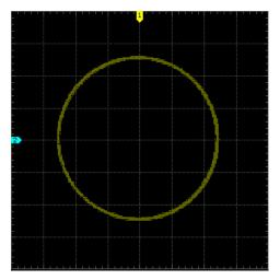
Observe the measurement result shown in the figure above. According to the measurement schematic diagram of the phase deviation (as shown in Figure 3-2), A/B (C/D) = 1. Thus, the phase deviation angle θ=±arcsin1=90°.
