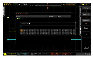
Figure 14-5 External Disk (To Create a New File)
