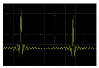
Figure 13-2 Sinc Function Waveform
