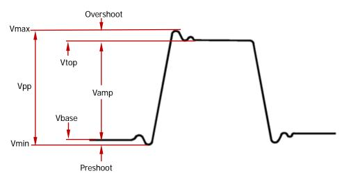
Figure 6-5 Voltage Parameters
