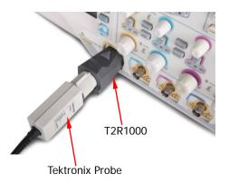
3. Connect the ground terminal of Tek probe to the ground terminal of the circuit. Connect the probe tip of Tek probe to the test point of the circuit under test.
