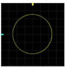
4. According to the phase deviation measurement principle diagram and the measurement result in the figure above, it can be calculated that  $\frac{A}{B}(\frac{C}{D}) = 1$ . Therefore, the phase deviation angle  $\theta = \pm \arcsin 1 = \pm 90^{\circ}$ .
