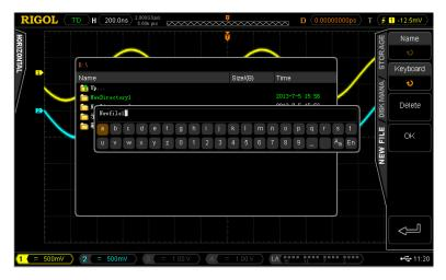
This oscilloscope supports Chinese/English input method. The filename or folder name can contain letters, numbers, underscores, spaces and Chinese characters and the length of the characters is limited to 31 bytes (one Chinese character occupies two bytes). Please input the desired name to create a new file or folder by referring to "English Input Method" and "Chinese Input Method"
