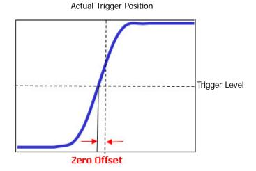
MSO4000/DS4000 allows users to set a delay time to calibrate the zero offset of the corresponding channel.
