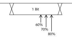
Press **Sample Point** and turn the multi-function knob  $\checkmark$  to adjust this parameter with a step of 1%. The default is 50%. The range is from 5% to 95%.
