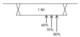
Press **Sample Point** and turn the multi-function knob  $\checkmark$  to adjust this parameter with a step of 1%. The default is 50%. The range is from 5% to 95%.
