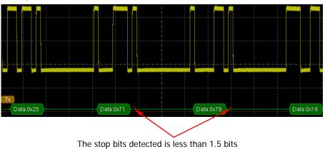
**Note:** When end of frame error and check error occur at the same time, two error marks will be displayed.
