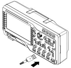
Figure 1-6 To Connect the Passive Probe
