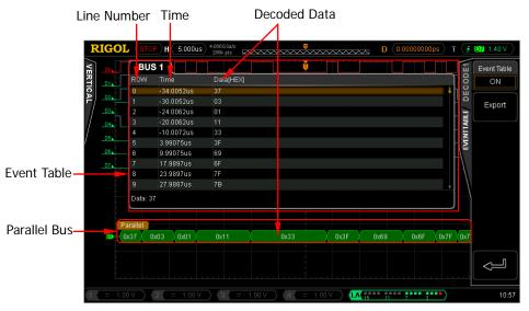
Figure 8-2 Parallel Decoding
