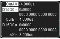
You can use cursor to perform manual measurement on the waveform of the LA channel following the steps below.
