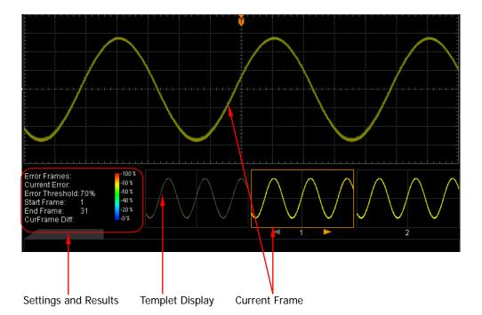
In the waveform recording menu (**Mode** is set to "Analyze"), you can set the related parameters of waveform analysis, execute the analysis operation and view the analysis results according to the instructions below.
