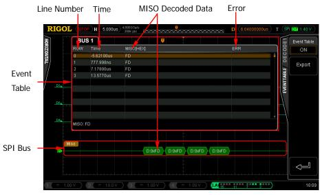
Figure 8-5 SPI Decoding
