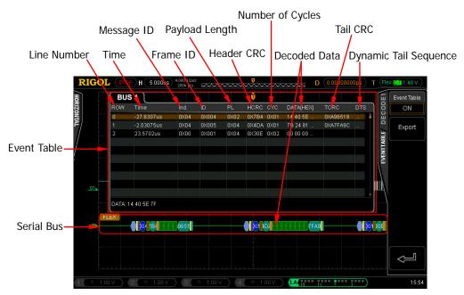
Figure 8-7 FlexRay Decoding
