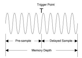
The relation of the memory depth, sample rate and waveform length fulfills the equation below:
