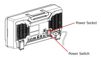
Figure 1-5 To Connect to Power Supply
