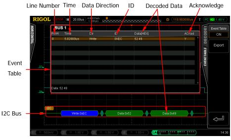
Figure 8-4 I2C Decoding
