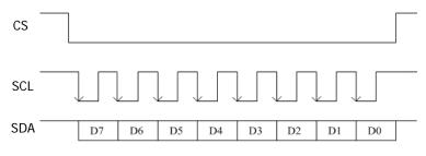
Figure 5-4 SPI Bus Sequence Chart
