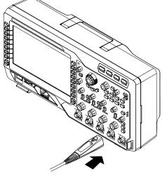
Figure 1-7 To Connect the Active Probe
