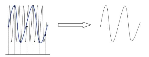
**3. Waveform Leakage:** when the sample rate is too low, the waveform rebuilt from the sample data does not reflect the actual signal completely.
