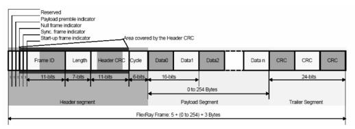
Figure 5-7 Frame Format of FlexRay Bus
