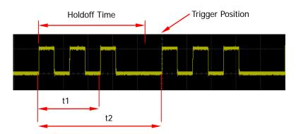
Press **MENU** (in the trigger control area (TRIGGER) at the front panel)  $\rightarrow$  **Setting**  $\rightarrow$  **Holdoff**; then, turn the multi-function knob  $\checkmark$  or the inner knob of the navigation knob to modify the holdoff time at a relatively smaller step or turn the outer knob of the navigation knob to adjust the holdoff time at a relatively larger step until the trigger becomes stable. The adjustable range is from 100 ns to 10 s. The default is 100 ns.
