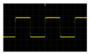
Figure 1-10 Probe Compensation Signal (Square Waveform)
