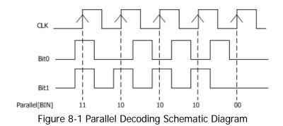
Press **Decode1**  $\rightarrow$  **Decode**, turn the multi-function knob  $\checkmark$  to select "Parallel" and press the knob. You can also press **Decode** continuously to switch to "Parallel".
