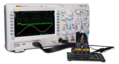
Figure 1-8 To Connect the Logic Probe
