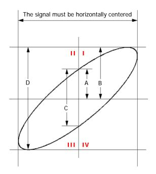
According to  $sin\theta = \frac{A}{B}$  or  $\frac{C}{D}$  (wherein,  $\theta$  is the phase deviation angle between the channels; the definitions of A, B, C and D are as shown in the figure above), you can calculate the phase deviation angle.
