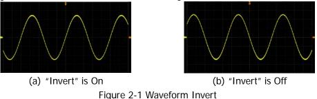
**Note:** Turning waveform invert on will change the results of math operations and waveform measurements.
