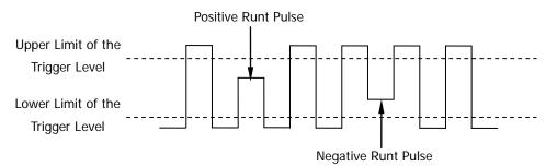
Press **MENU** (in the trigger control area (TRIGGER) at the front panel)  $\rightarrow$  **Type**, turn the multi-function knob  $\heartsuit$  to select "Runt" and press the knob. You can also press **Type** continuously to switch to "Runt" trigger.
