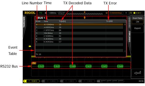
Figure 8-3 RS232 Decoding
