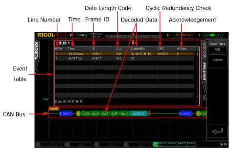
Figure 8-6 CAN Decoding
