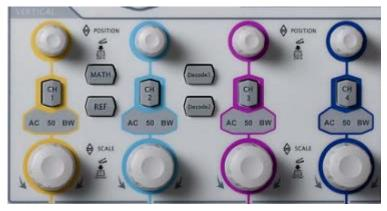
• CH1, CH2, CH3, CH4: analog input channel switches.
