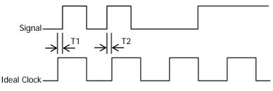
Figure 7-1 Digital Bus Jitter Schematic Diagram
