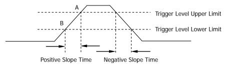
Figure 5-1 Positive Slope Time/Negative Slope Time
