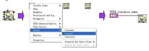
Separately connect "VISA resource name" with "VISA resource name out" and "error out" with "error in" of all the functions. See the figure below.
