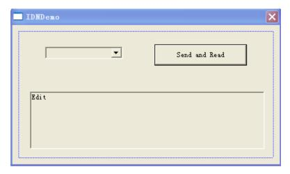
Respectively add two variables m\_combox and m\_receive for the controls of Combo Box and Edit Box. See the figure below.
