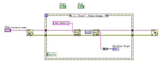
8. Right-click the "selector label" and choose "Edit Events Handled by This Case" or "Add Event case" to add events respectively for each button. Press "Start" to capture waveform and "Stop" to exit the program.
