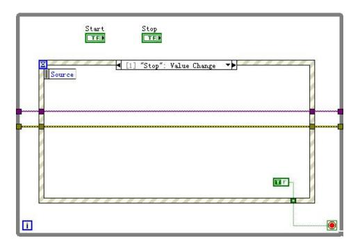
**10.** Change the input tunnel of VISA resource name and errors into **"Shift Register"** to finish creating program.
