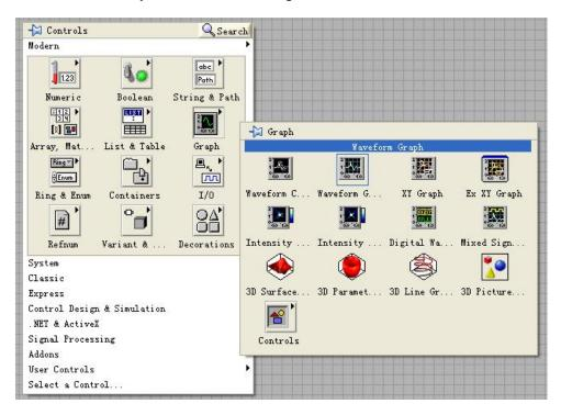
6. open Block Diagram; right-click and choose Programming → String → String/Array/Path and select "String To Byte Array"; then, use this function to connect "read buffer" on "VISA Read" function with the Waveform Graph.
