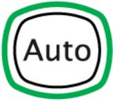
Press this key to turn on the waveform auto setting function. The oscilloscope will automatically adjust the vertical scale, horizontal time base and trigger mode according to the input signal to realize optimum waveform display. Note that auto setting requires that the frequency of the signal under test should be no lower than 50 Hz, the duty cycle be greater than 1% and the amplitude be at least 20 mVpp.
