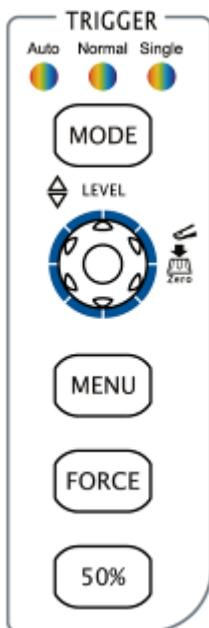
**MODE**: press this key to switch the trigger mode to **Auto**, **Normal** or **Single** and the corresponding state light backlight of the current trigger mode would be illuminated.
