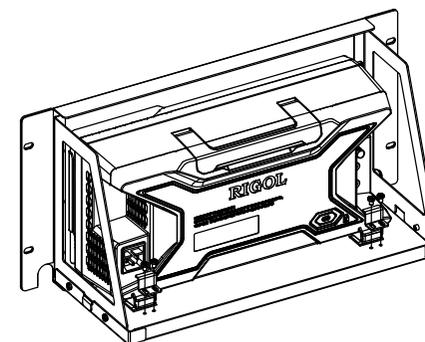
(4). Load into the machine cabinet: mount the rack with the instrument fixed to it into a standard 19-inch machine cabinet with four M6 screws and four M6 square nuts.
