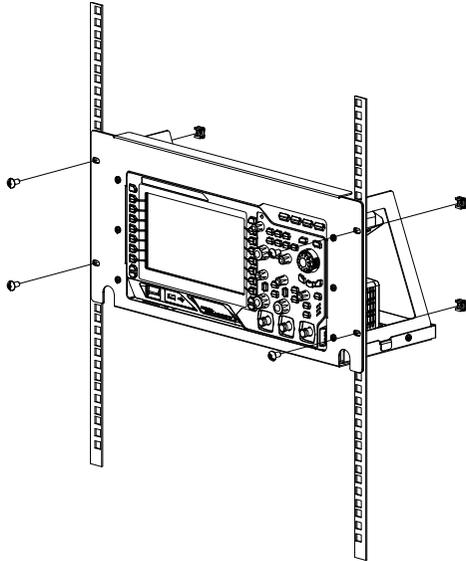
(5). Post-installation notice: the rack occupies a height of 5U. The holes pointed out by the arrows are installation holes. Note that they should be aligned with during installation.
