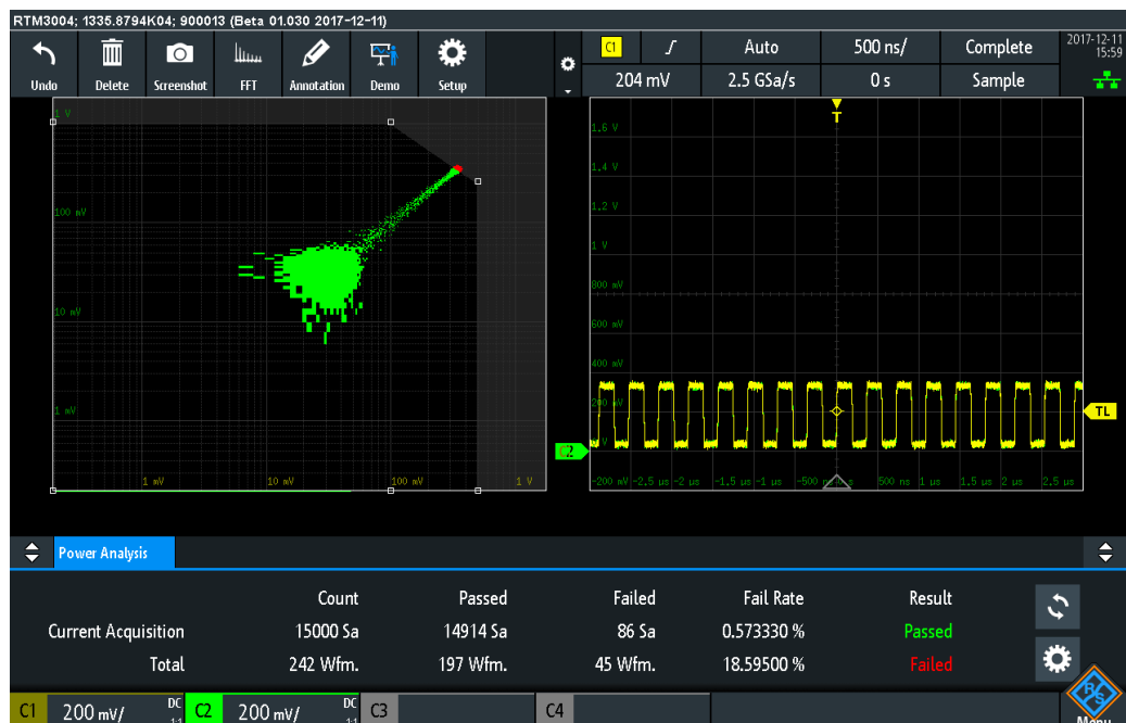
Figure 14-14: Results of the SOA power measurement
