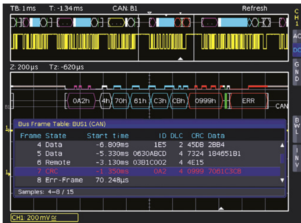
Figure 11-17: Example of a CAN bus table
