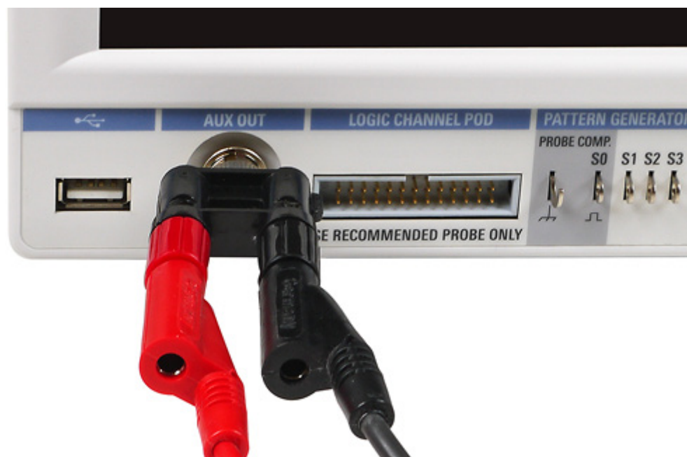
Figure 6-14: BNC/banana adapter connected to [Aux Out]
