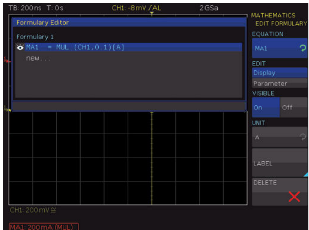
Figure 6-10: Definition of the current equation
