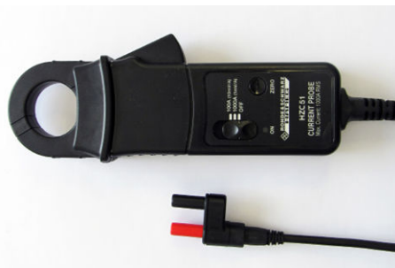
Figure 4-7: R&S HZC51 clamp-on current probe
