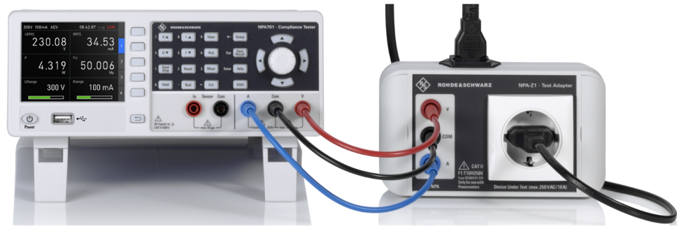
Figure 4-4: R&S NPA-Zx to R&S NPA measurement setup
