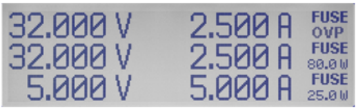
Figure 5-6: Overvoltage protection (example R&S HMP2030)
