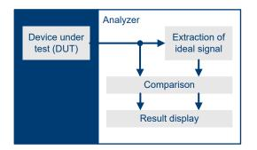
Figure 17-1: Demodulation principle
