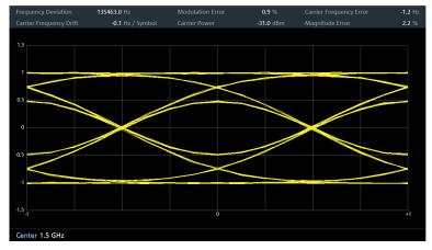
Figure 17-2: Eye diagram of a 2FSK signal
