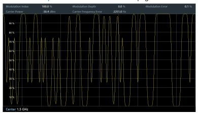
Figure 17-4: Modulation depth of a 2ASK signal
