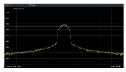
Figure 14-21: Display line at -38 dBm
