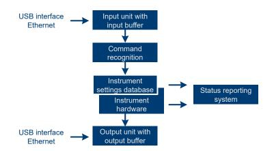
Figure 19-4: Instrument model in case of remote control
