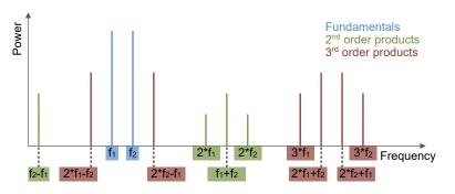
Figure 14-4: Overview of intermodulation products
