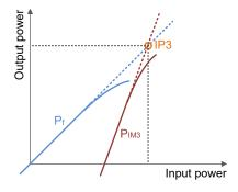
The third order intermodulation (TOI) measurement analyzes the intermodulation products that occur at the output of the DUT and calculates the third order intercept point. The IP3 is the theoretical intercept point of the DUTs desired output level and the level of the intermodulation products. It is thus a measure of the DUTs linearity.
