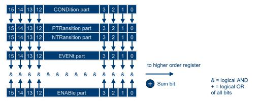
Figure 19-5: Model of the status register
