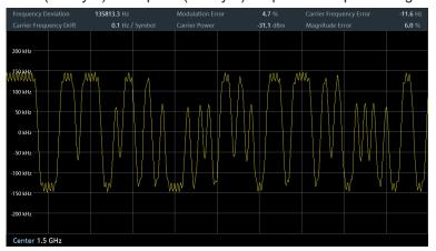
Figure 17-5: Modulation deviation of a 2FSK signal
