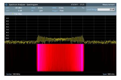
This provides a high contrast between signal parts that are above the noise floor, and the noise floor, which is drawn in black.
