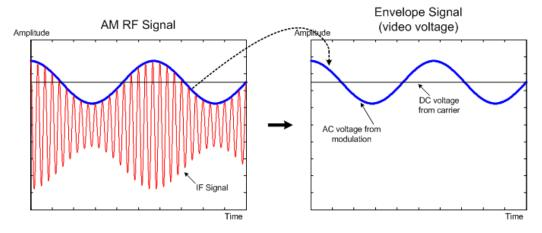
Figure 14-11: Video voltage of an AM signal
