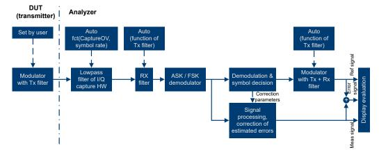
Figure 17-8: Block diagram of measurement filter
