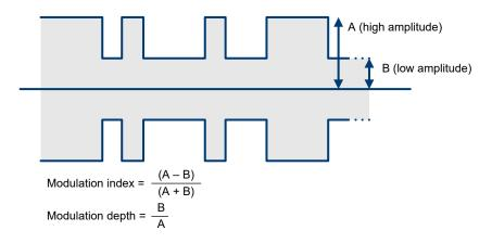
Figure 17-7: Calculation of modulation index and depth
