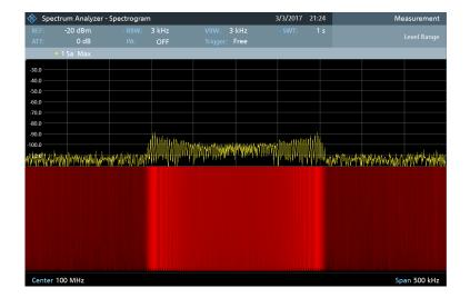
Therefore you can adjust the color map to the overall shape of the signal you are measuring. Let us say, for example, that the signal has an amplitude range of about 30 dB with the maximum amplitude at about -80 dBm and the minimum amplitude at about -120 dBm. With the default settings, the spectrogram is made up exclusively of red colors and it is not easy to distinguish amplitude levels. That is because the purple color shades are completely out of range.
