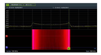
Figure 14-6: Time lines and markers in the spectrogram
