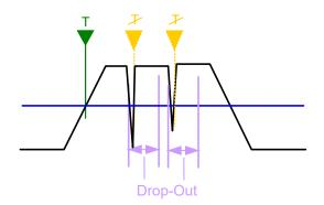
Figure 6-46: Effect of the trigger drop-out time
