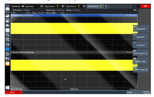
Figure 4-11: Inserting a Real/Imag diagram for I/Q analysis
