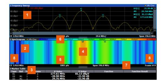
Figure 6-55: Screen layout of the spectrogram result display
