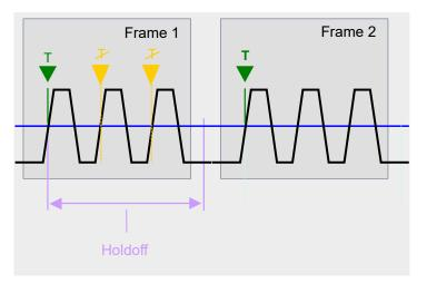
Figure 6-48: Effect of the trigger holdoff
