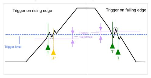
Figure 6-45: Effects of the trigger hysteresis
