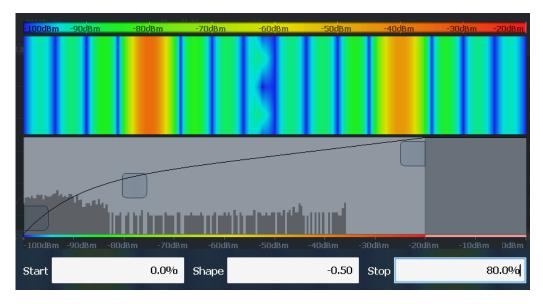
Figure 6-58: Spectrogram with non-linear color curve (shape = -0.5)
