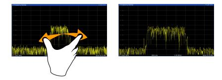
Figure 4-24: Spreading
