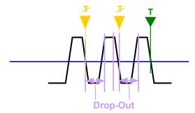
Figure 6-47: Trigger drop-out time for falling edge trigger
