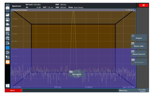
Figure 4-6: Adding a Spectrogram to the display
