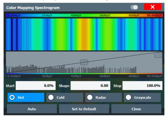
Figure 6-57: Spectrogram with (default) linear color curve shape = 0
