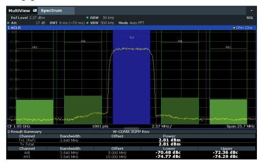
Figure 6-23: Measuring the relative adjacent channel power on a W-CDMA uplink signal
