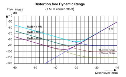
Figure 6-38: Intermodulation-free range as a function of level at the input mixer and the set resolution bandwidth
