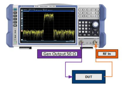
Figure 6-42: Test setup using the internal generator
