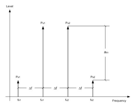
Figure 6-36: Intermodulation products Ps1 and Ps2
