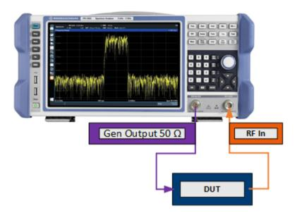
Figure 6-20: Test setup for compression point measurement using an internal generator
