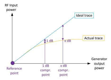
Figure 6-21: Compression point calculation
