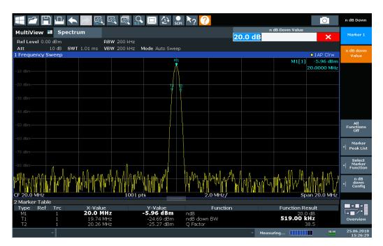
Figure 6-49: n dB down marker function
