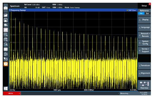
Figure 4-4: Calibration signal as RF input
