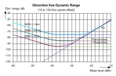
Figure 6-39: Intermodulation-free dynamic range as a function of level at the input mixer and of the selected resolution bandwidth
