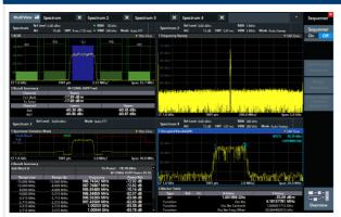
Configure your result windows the way you want. Display multiple measurement channels at once. Sequential channel updating allows e.g. parallel measurement of the spectrum, spectrogram and analog demodulation together with  $I/\Omega$  analysis.
