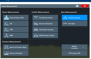
Fast and easy access to a wealth of measurement and marker functions in the base model, including spectrogram measurements and I/Q analysis. Quick configuration through clear menus and touchscreen operation.
