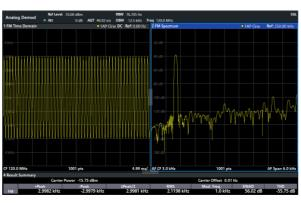
Frequency deviation measurement: display of modulation signal together with peak and RMS deviation, carrier frequency offset and carrier power
