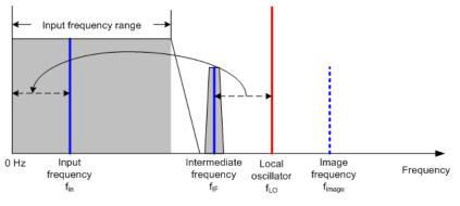
Figure 6-3: Mixing process
