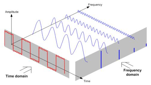
Figure 6-1: Visualization of time domain and frequency domain
