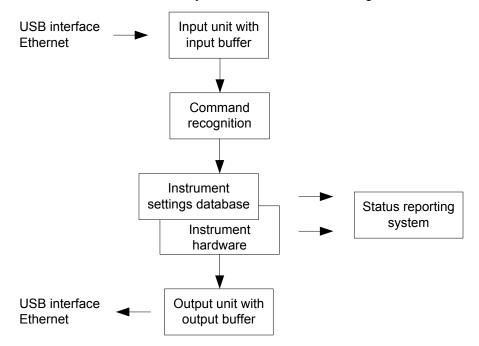
Figure 7-4: Instrument model in the case of remote control
