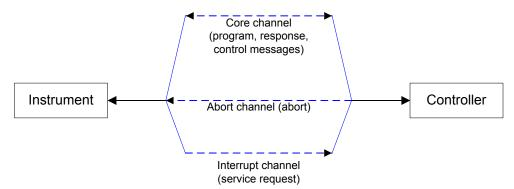
Figure 7-2: VXI-11 channels between instrument and controller
