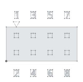
11: Channel 3 2: GND 3: Channel 2 4: GND 5: Channel 1 6: GND 7: Channel 0 2) Add female right-angle headers to the edge of your board, or vertical headers to mount the logic analyzer vertically to your board.
