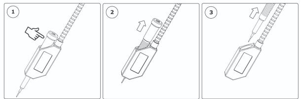
**Position the probe** - Place the probe foot on the base plate and the magnet will keep it in place.
